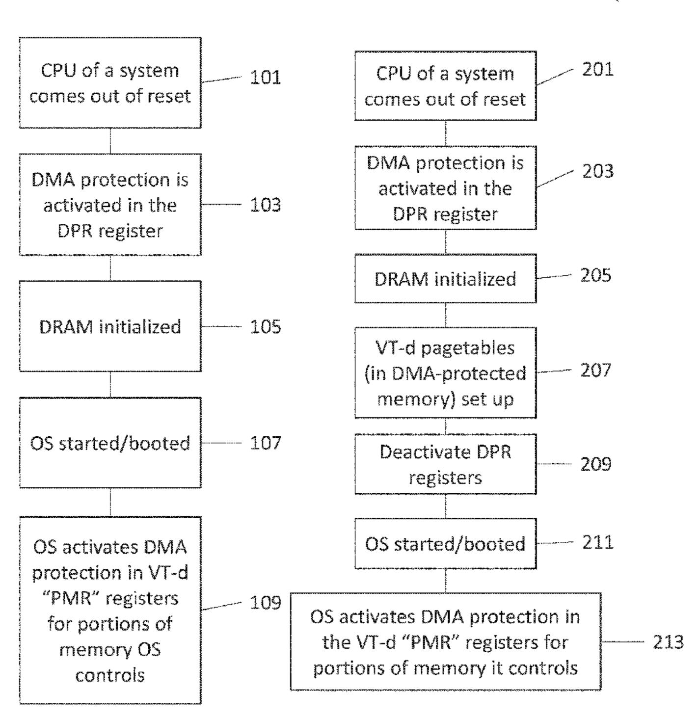
drivers and non-DMA related hardware initialization instructions, and using a memory management tool, allocating a first part of the physical memory, accessible by a device via the memory management tool, for use by data.
