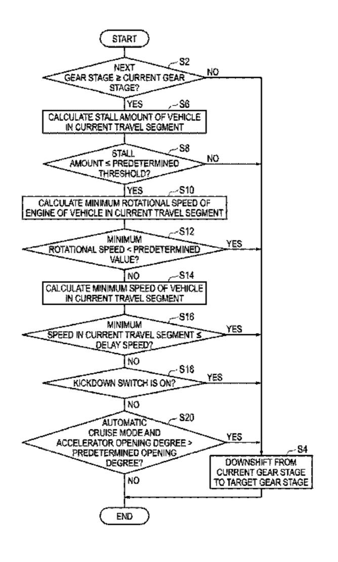
suppressed and the current gear stage is maintained. Even in a state in which downshifting is suppressed, if the state of the vehicle the satisfies a prescribed condition, then the shift control unit 17 controls shifting of the gear stage so as to downshift to the target gear stage without suppression of downshifting.
