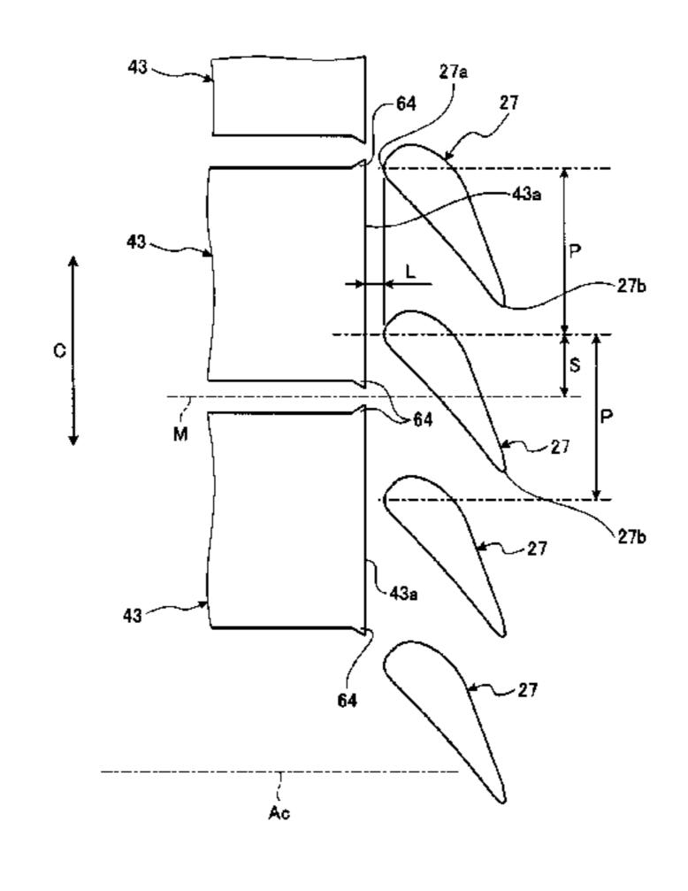
a pitch dimension of first stage vanes, and (S) is a circumferential dimension from an intermediate point between neighboring transition pieces to an upstream end of a first stage vane closest in the circumferential direction; and a ratio (L/P) is from 0.3 to 0.55, where (P) is the pitch dimension, and (L) is an axial dimension from a downstream end of the transition piece to the upstream end of the first stage vane.
