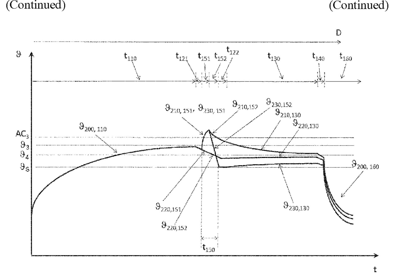
the third regions are cooled to a cooling stop temperature  $\vartheta$ s. The component is transferred into a second furnace, with a temperature lying below the AC3 temperature. There, the temperatures of the three different regions approximate one another.
