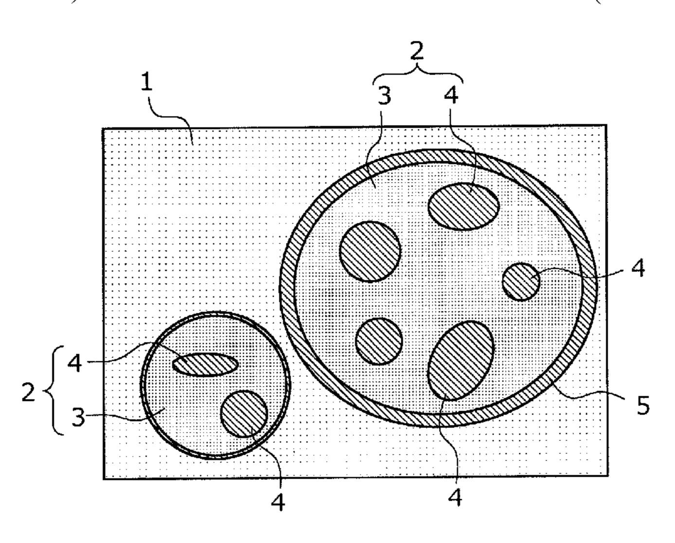
olefin-based thermoplastic elastomer having, as a skeleton, a copolymer of ethylene or propylene and an  $\alpha$ -olefin having 3-8 carbon atoms or a styrene-based thermoplastic elastomer having a styrene skeleton, and when a total of the continuous phase (A) and the dispersed phase (B) is taken as 100% by mass, a content of the dispersed phase (B) is 80% by mass or less.
