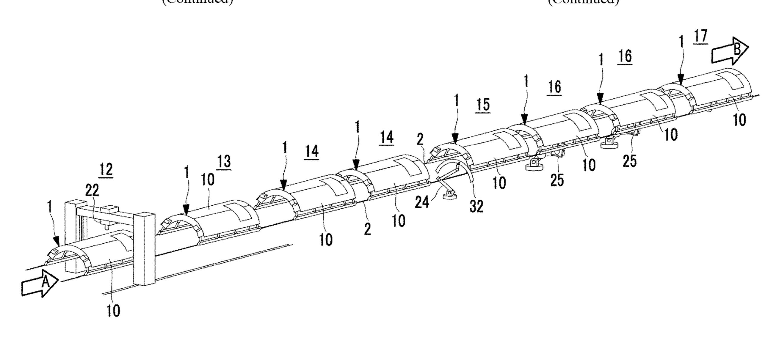
a rivet; a step in which the holding jig, which is holding the body panel of which the plate-like members have been joined to each other, is moved; and a step in which a frame that follows the curved shape of the body panel is joined, by a rivet, to the plate-like members of the body panel which is held by the holding jig which has been moved.
