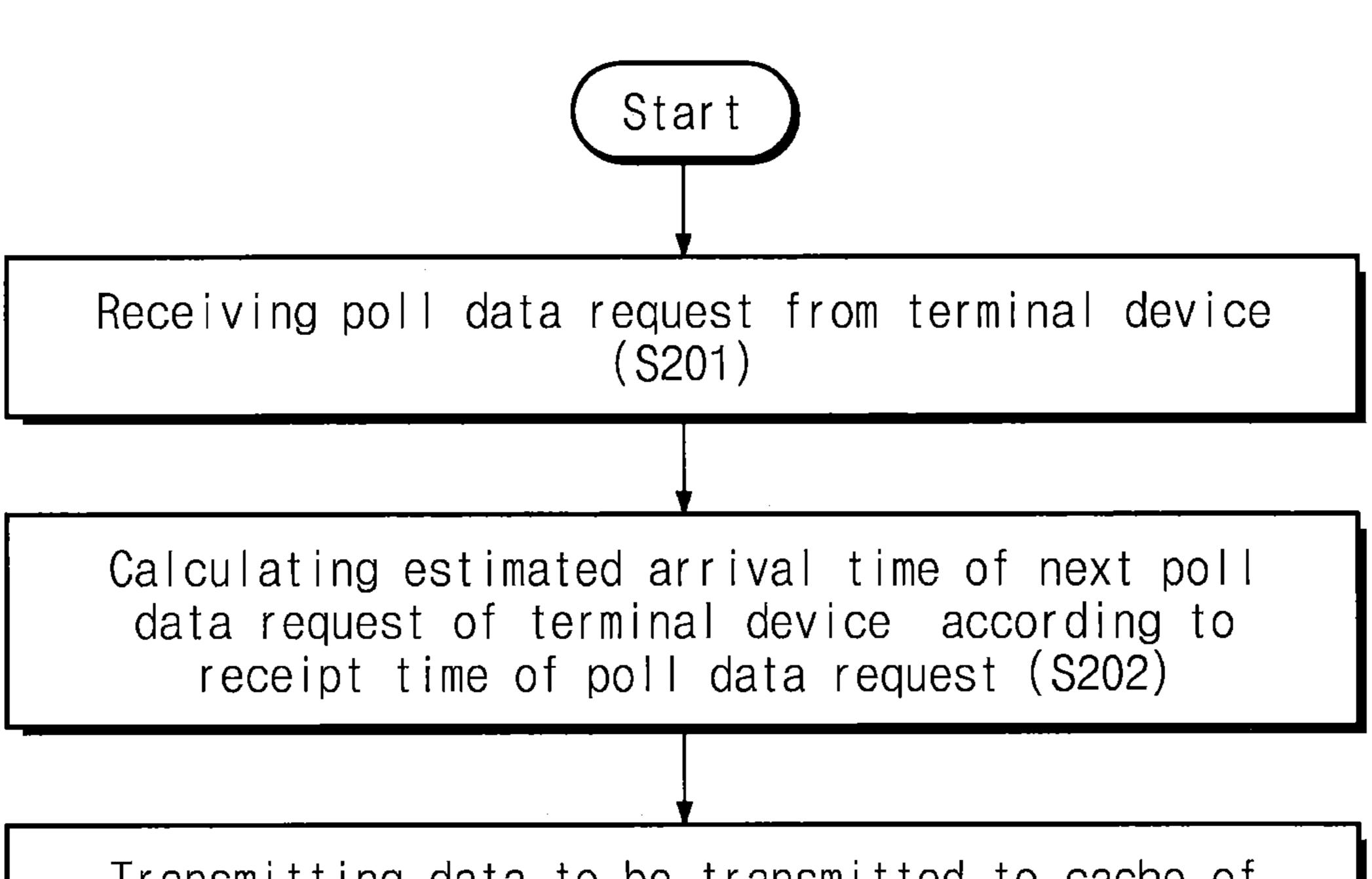
Transmitting data to be transmitted to cache of MAC layer module at time point which is predetermined time length ahead of estimated arrival time when there is data to be transmitted in network layer module (S203)
