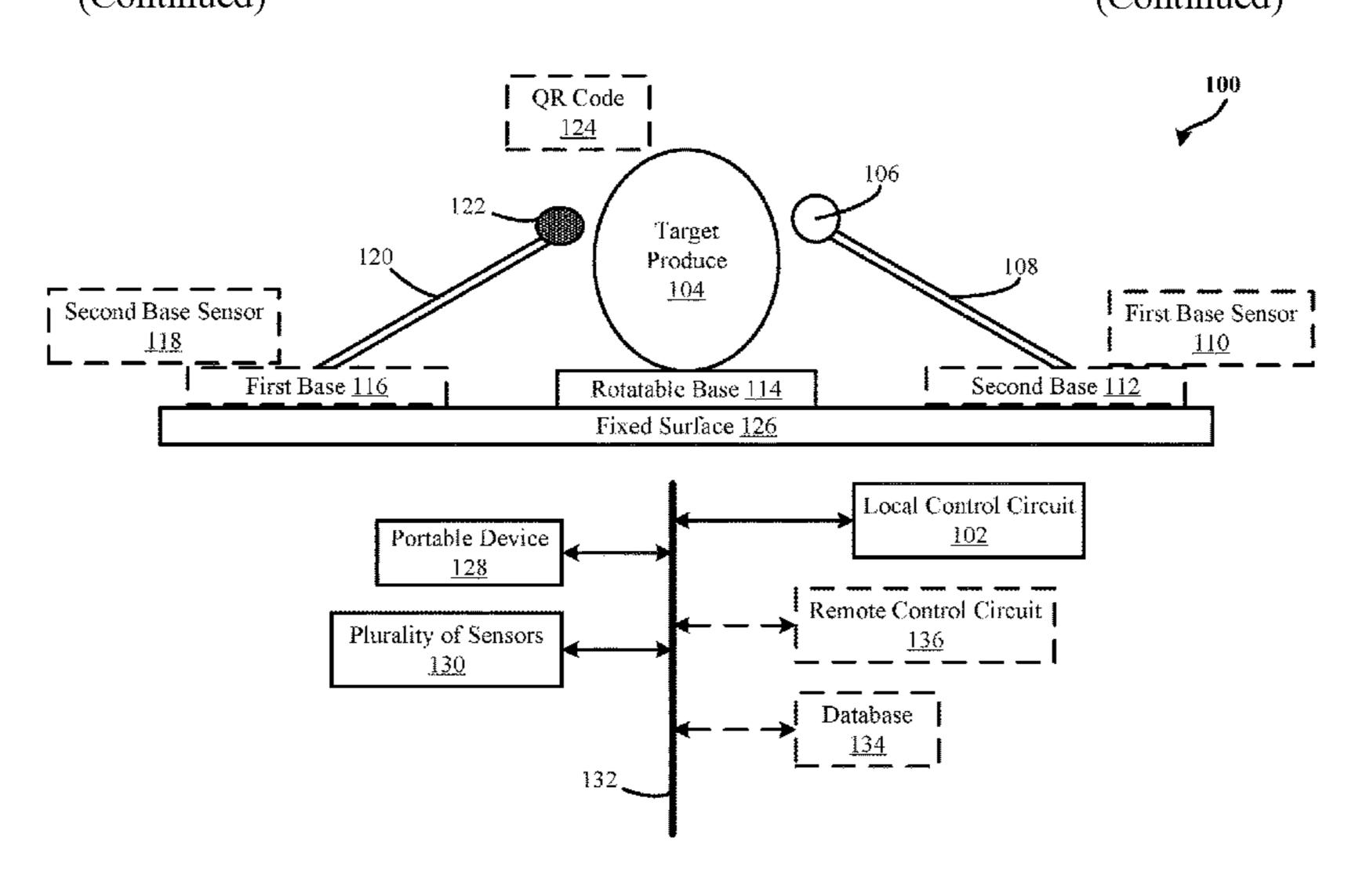
from the microphone. By one approach, the system includes a plurality of sensors and a portable device configured to provide a signal to the local control circuit to initiate the quality classification of the target produce.
