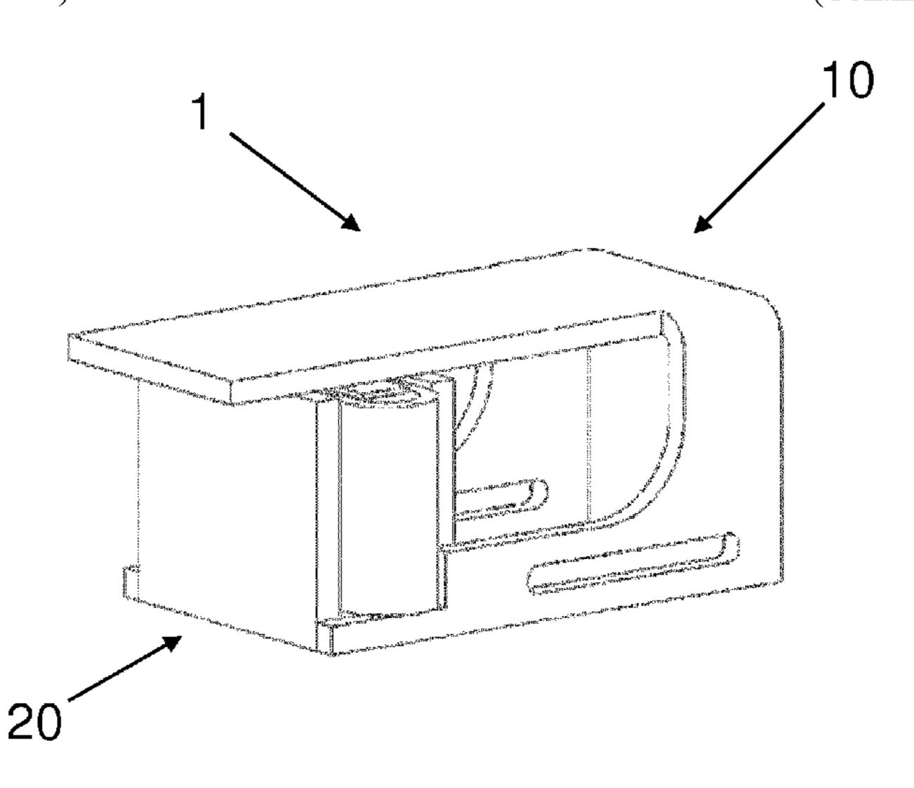
electromagnetic feedback actuator coupled to an operating element.
