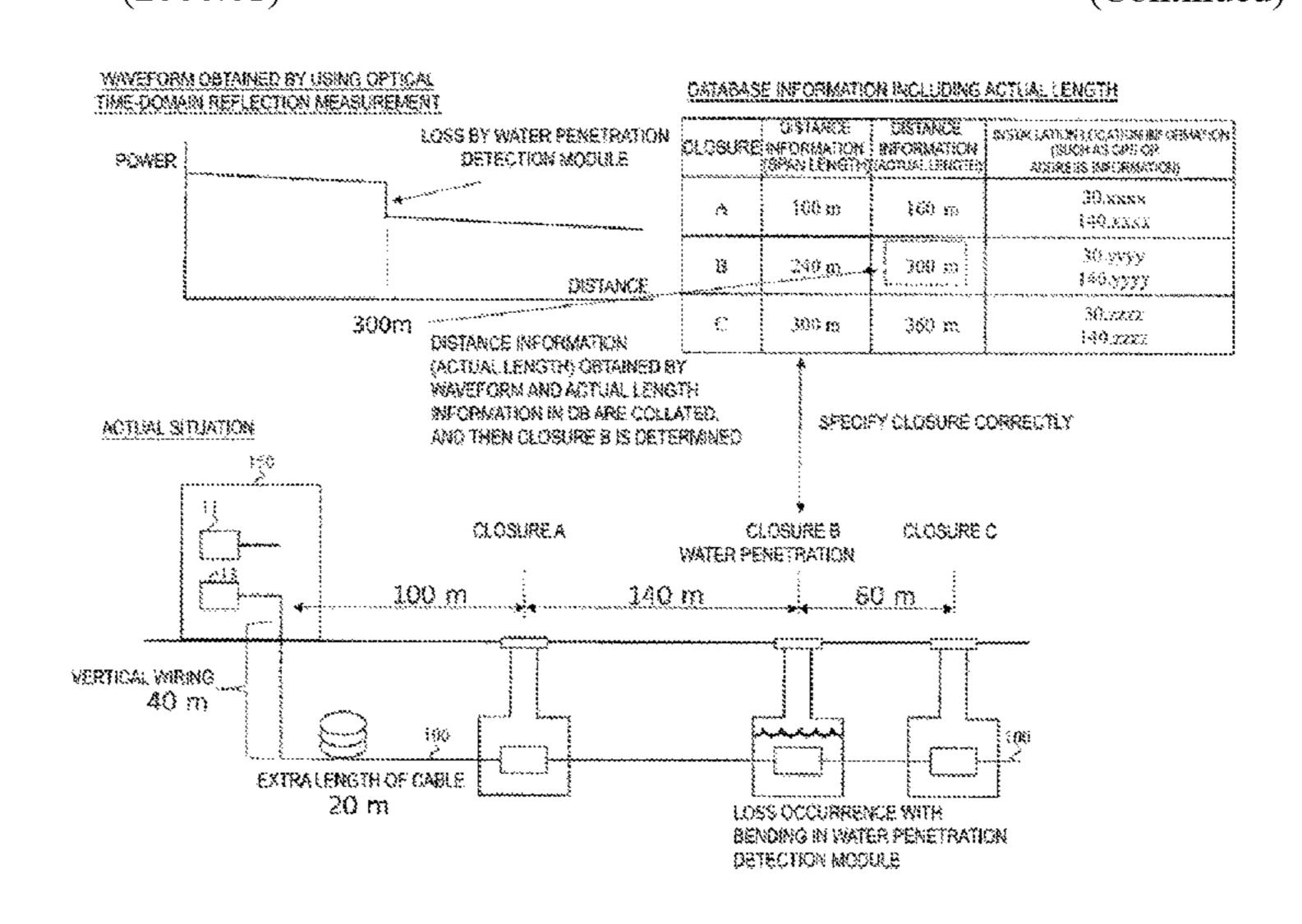
that is linked to a location of a point of abnormality on the optical fiber cable when an abnormality in the closure is detected with a low-sensitivity measurement technique.
