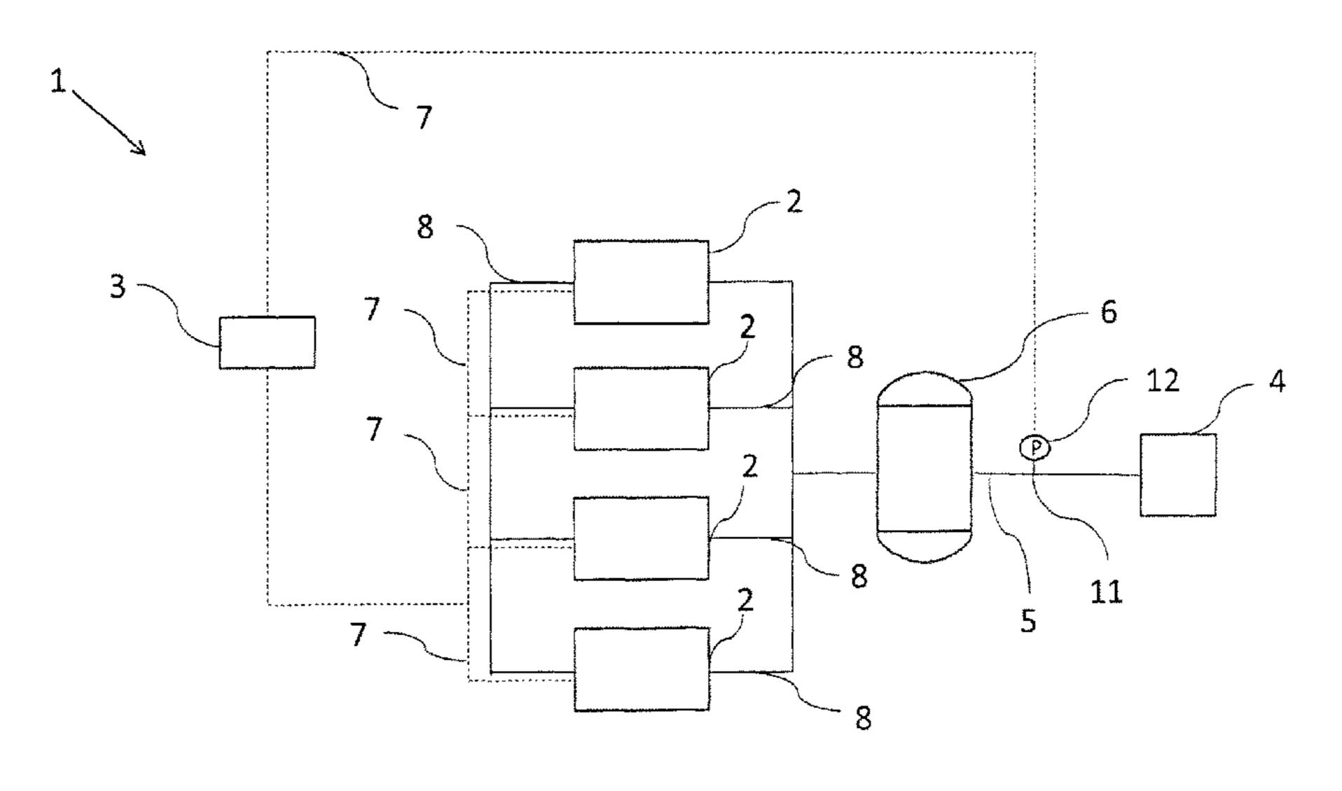
method further includes the steps of measuring the inlet pressure p1, comparing the measured inlet pressure p1 with a predetermined pressure value p0, and if p1 is higher than p0, starting the secondary vacuum pump at a first predetermined startup load  $S_{startup,1}$  if it includes a fixed speed motor, and/or starting the secondary vacuum pump at a second predetermined startup load  $S_{startup,2}$ , if it includes a variable speed motor.
