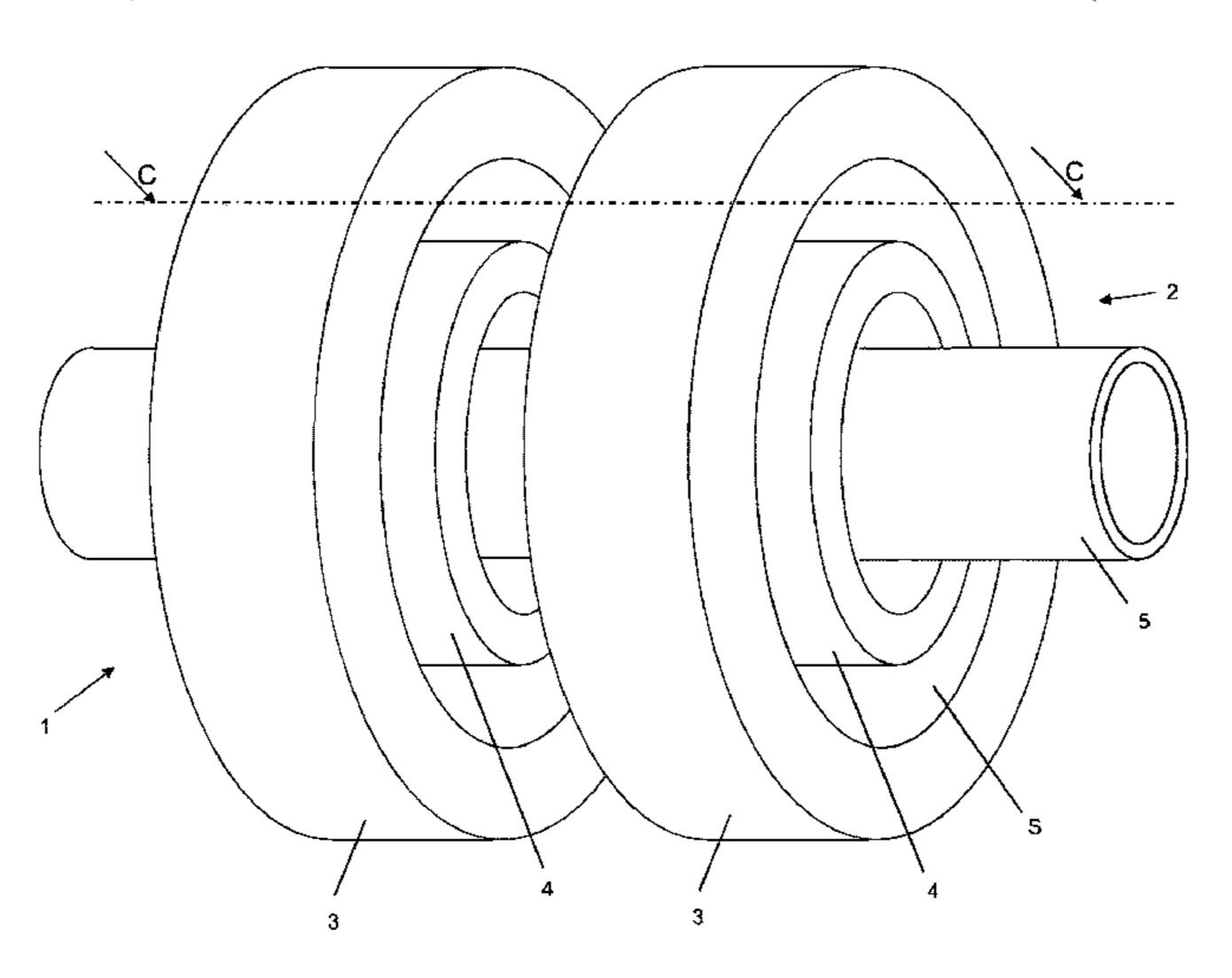
coil rings (3, 4), whereby a fluid (L), especially an air stream, that serves to cool the coil device (1, 2) can flow through the space.
