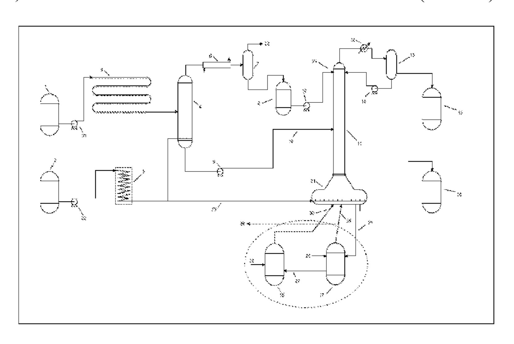
catalyst selected from the lanthanide series are added in a reactor to afford dialkyl carbonate. The rare earth metal catalyst is selected from samarium, cerium, lanthanum, neodymium, ytterbium, europium and gadolinium. Ammonia is added to a portion of the reaction mixture to precipitate the catalyst and the separated deactivated catalyst is dissolved in acid to afford regenerated catalyst, e.g., in triflic acid in the case of samarium triflate catalyst.
