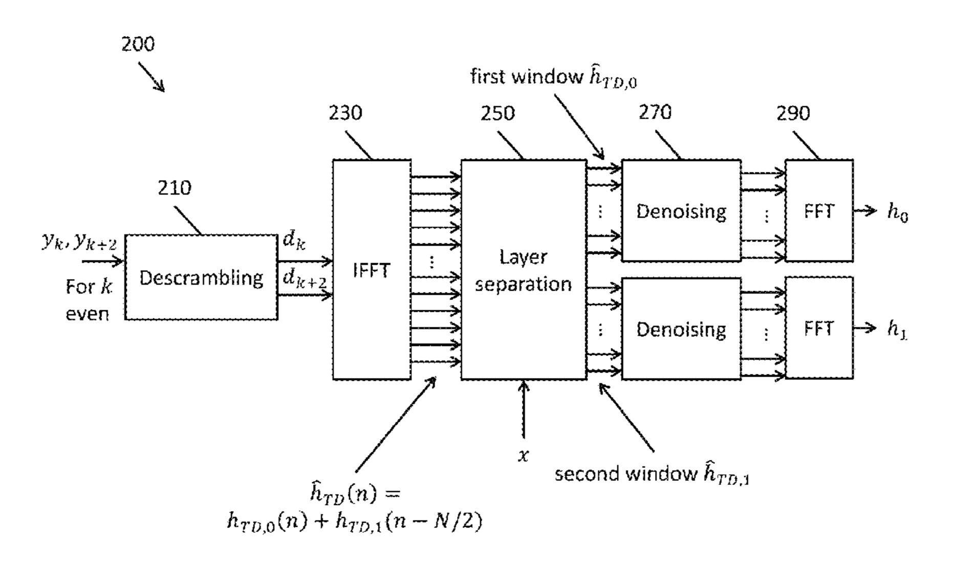
sampling window in accordance with a size of the inverse fast Fourier transform; extracting one or more first layers from the samples in the first time domain sampling window; and extracting one or more second layers from the samples in the second time domain sampling window.
