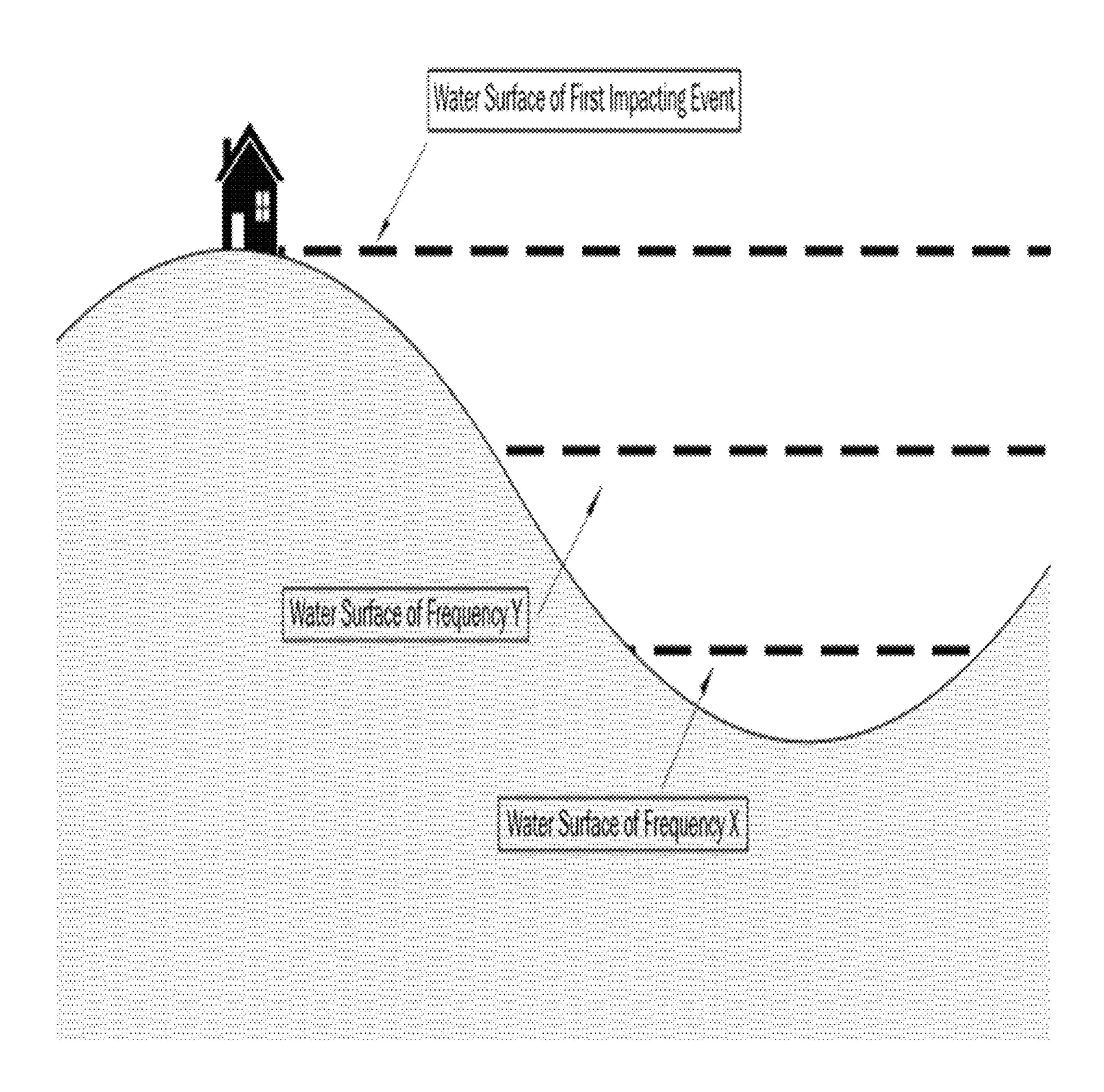
Fig. 9 Vertical criterion of a Threshold (First Impacting) Event "touching" a location and a structure
