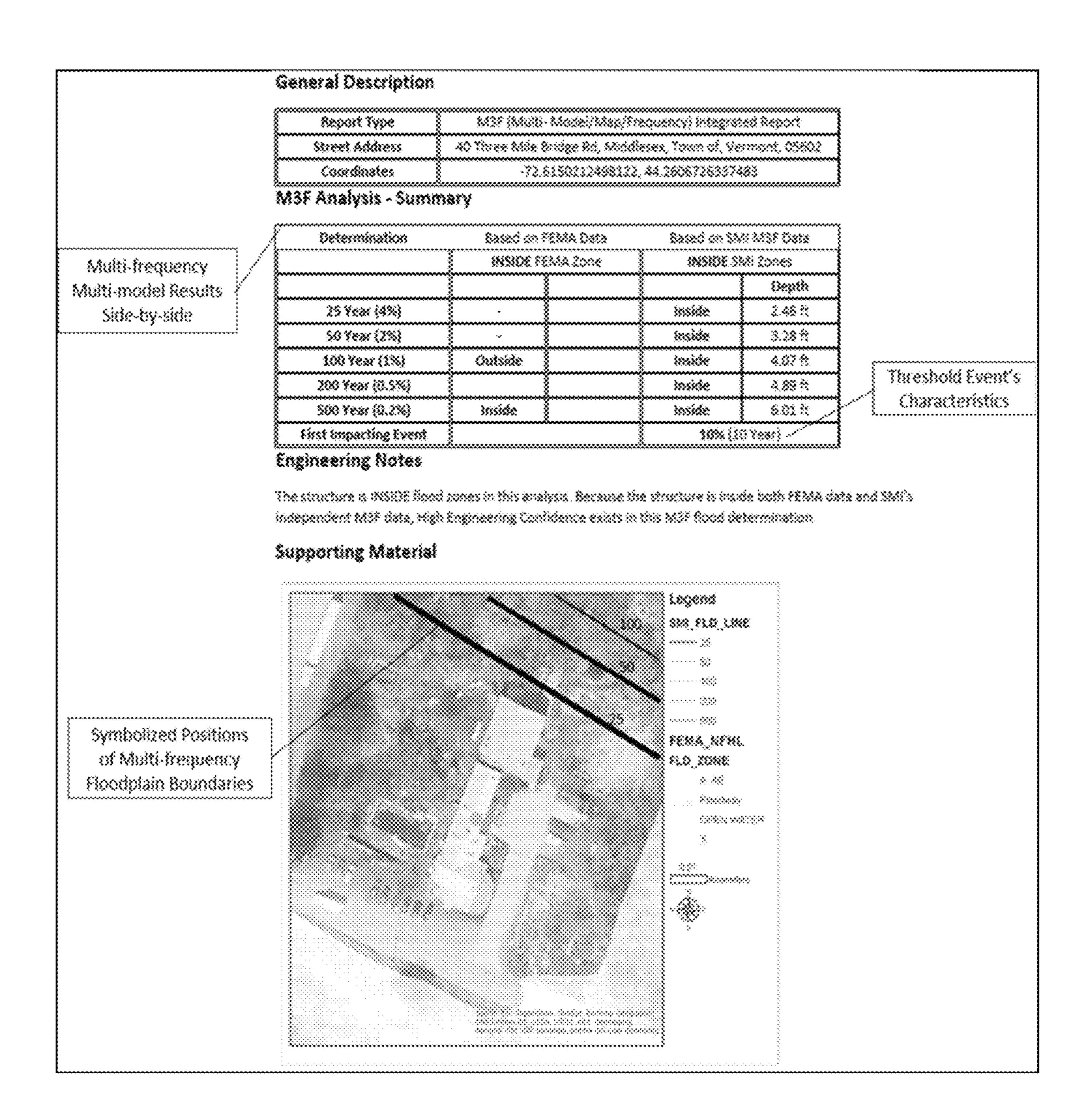
Fig. 12 Key parts of a M3F report with a Threshold (First Impacting) Event
