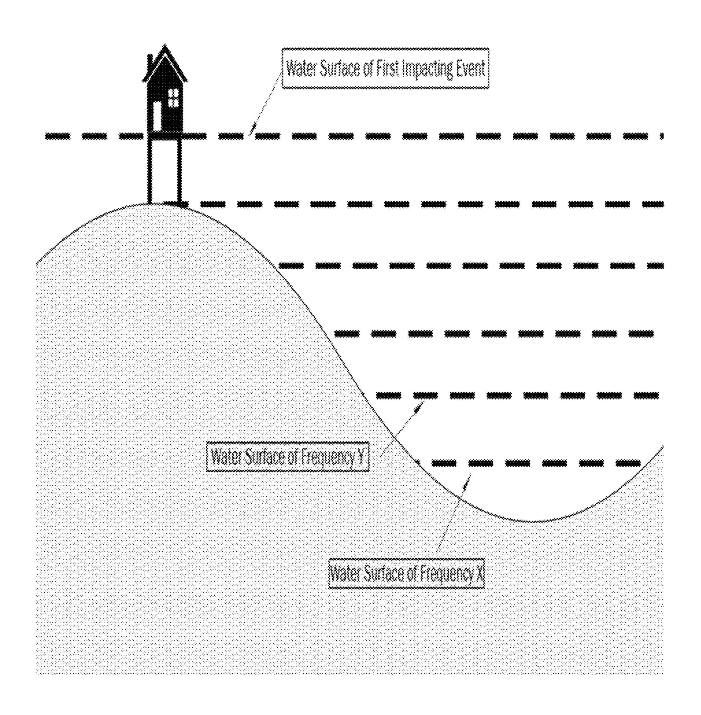
Fig. 10 Vertical criterion of a Threshold (First Impacting) Event "touching" a location and an Elevated Structure
