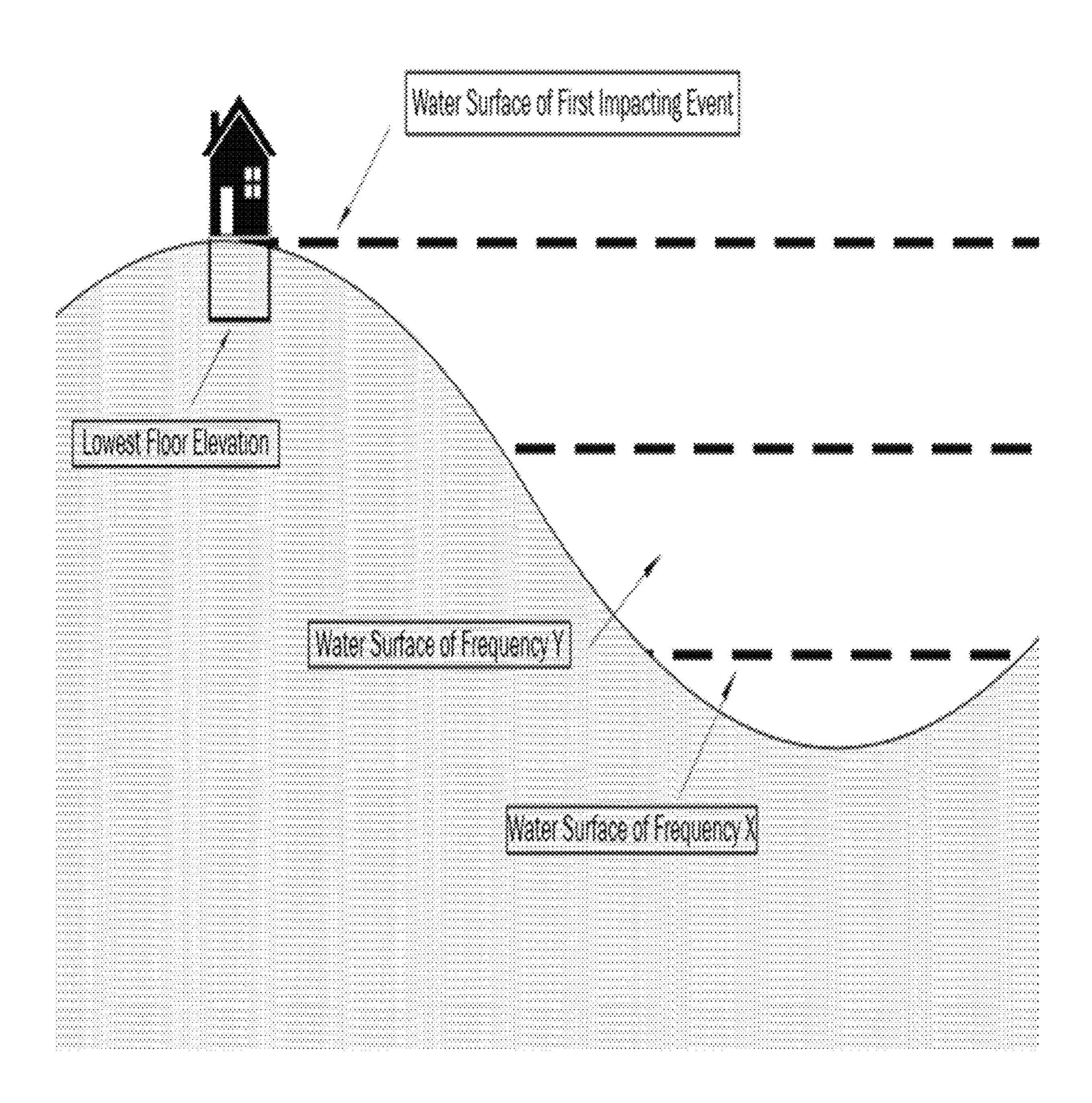
Fig. 11 Vertical criterion of a Threshold (First Impacting) Event "touching" a location and a structure with a basement
