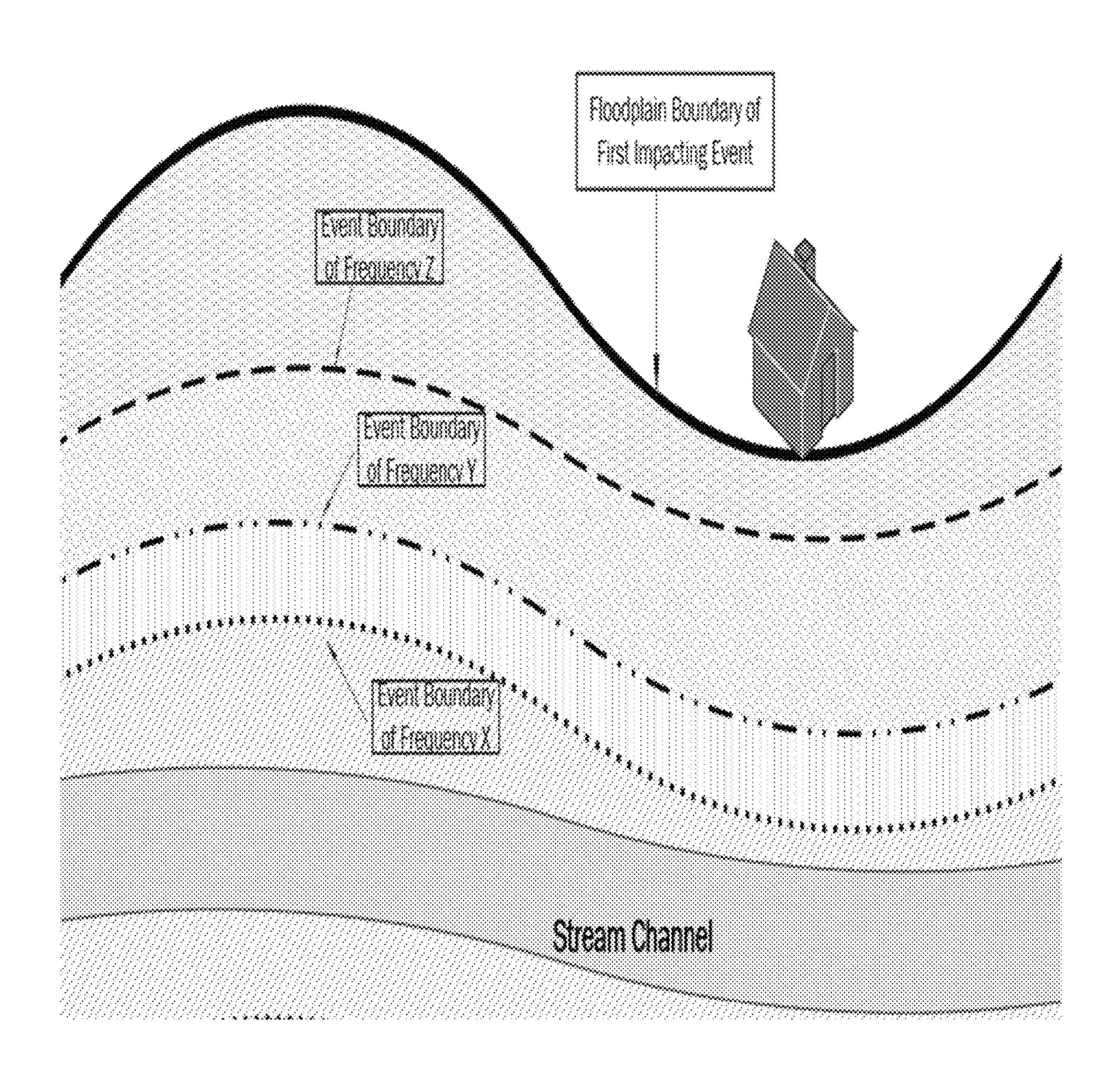
Fig. 8 Horizontal criterion of a Threshold (First Impacting) Event "touching" a location and a structure
