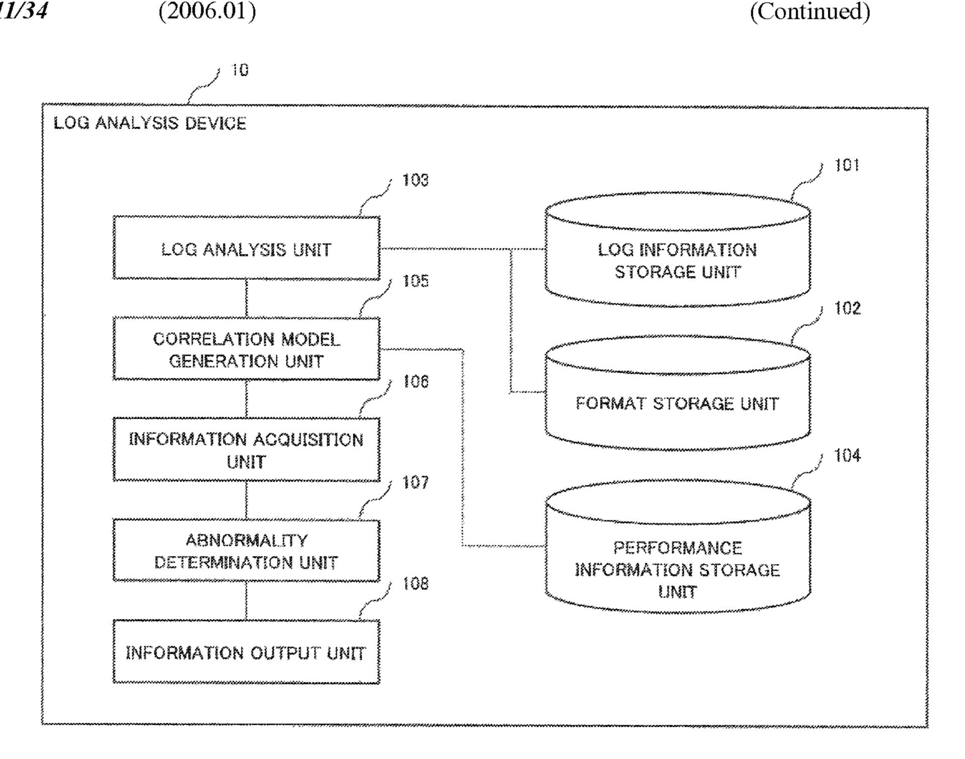
and a determination unit that determines existence of an abnormality in the monitored target based on the correlation model.
