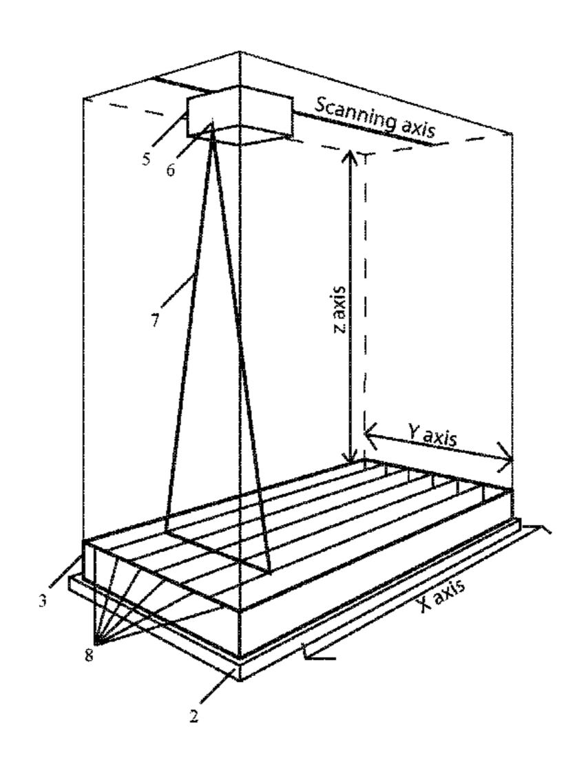
dimensional shape and appearance of drill core samples, such as planar discontinuities including orientation marks on the drill core samples.
