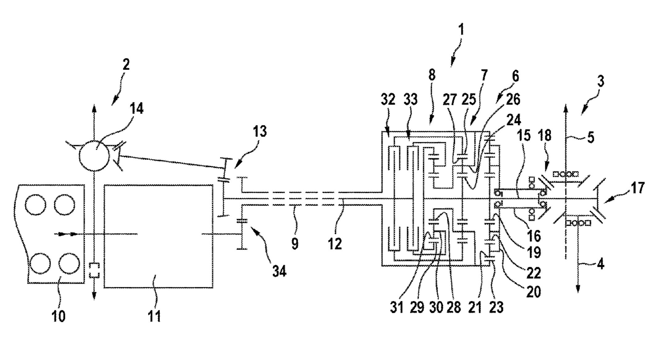
first connecting shaft and the second connecting shaft in a torque-splitting manner.
