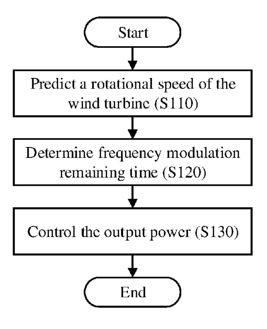
output power used for the primary frequency modulation without affecting a recovery of the wind turbine after the primary frequency modulation; controlling the output power based on the determined frequency modulation remaining time.
