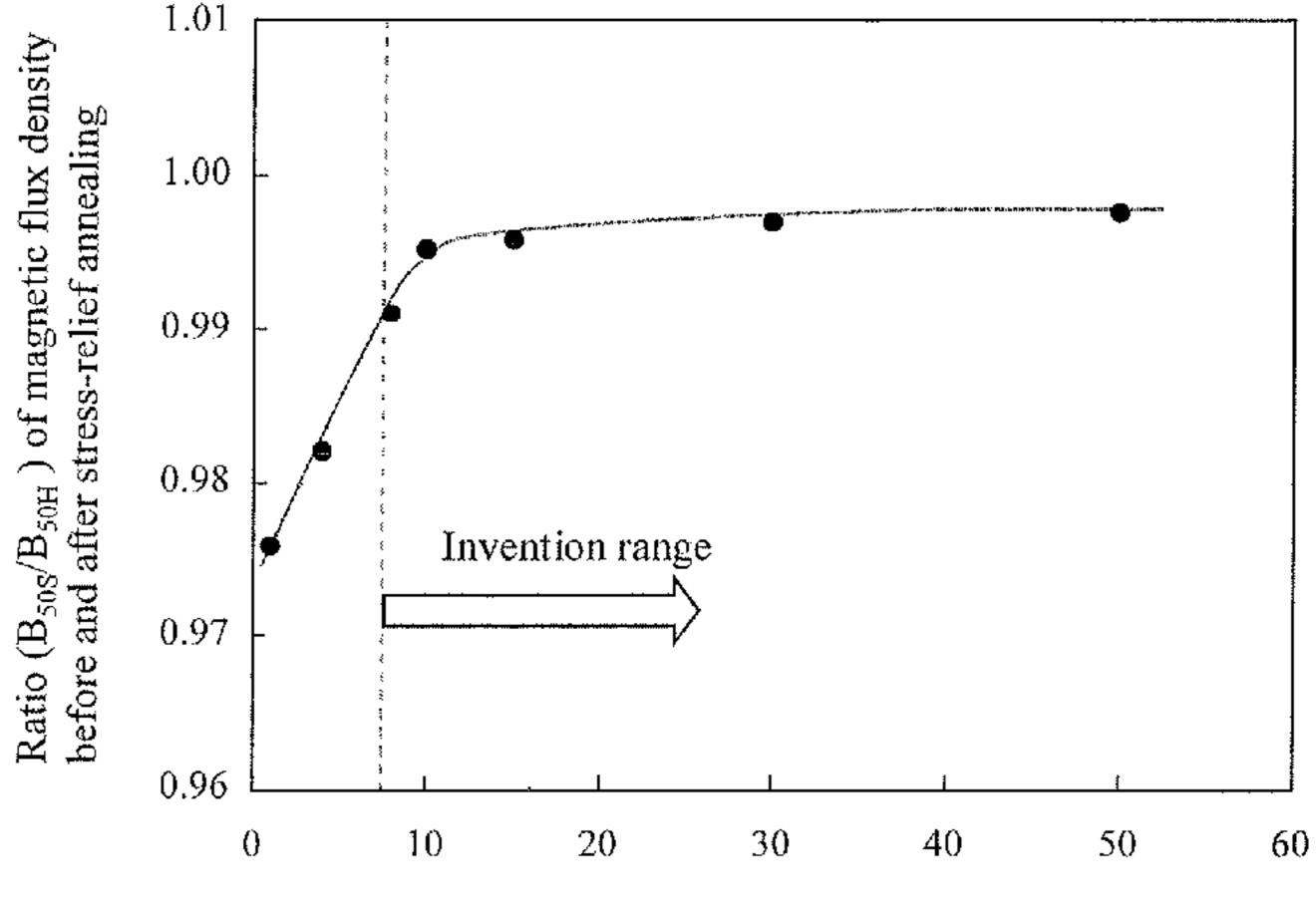
Heating rate in stress-relief annealing (°C/min)
