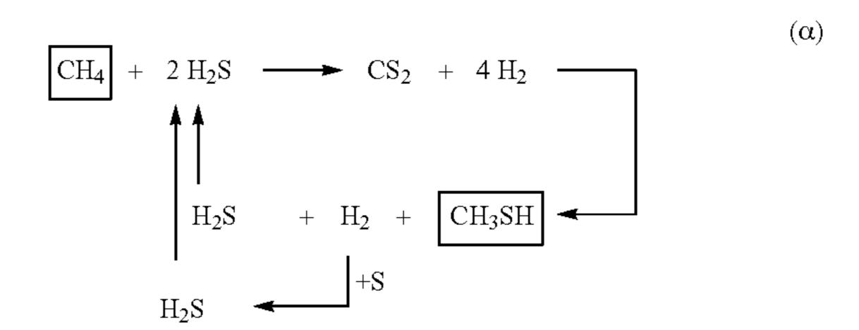
According to a variant of the process of the invention, the sulphur may be introduced in the first step (step a)). The balanced reaction may then be written in accordance with scheme (7):
