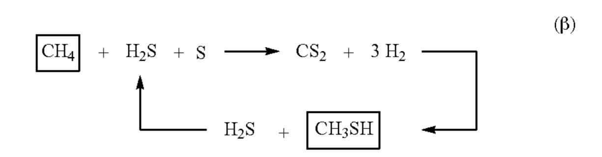
All of the above reactions involve methane (CH<sub>4</sub>) as initial hydrocarbon charge, but the process of the invention may be carried out in a similar manner from any type of hydrocarbon charge. For a hydrocarbon charge of type  $C_aH_{2b}$ , the general equation corresponding to the reaction of 5 the first step (step a)) then becomes:
