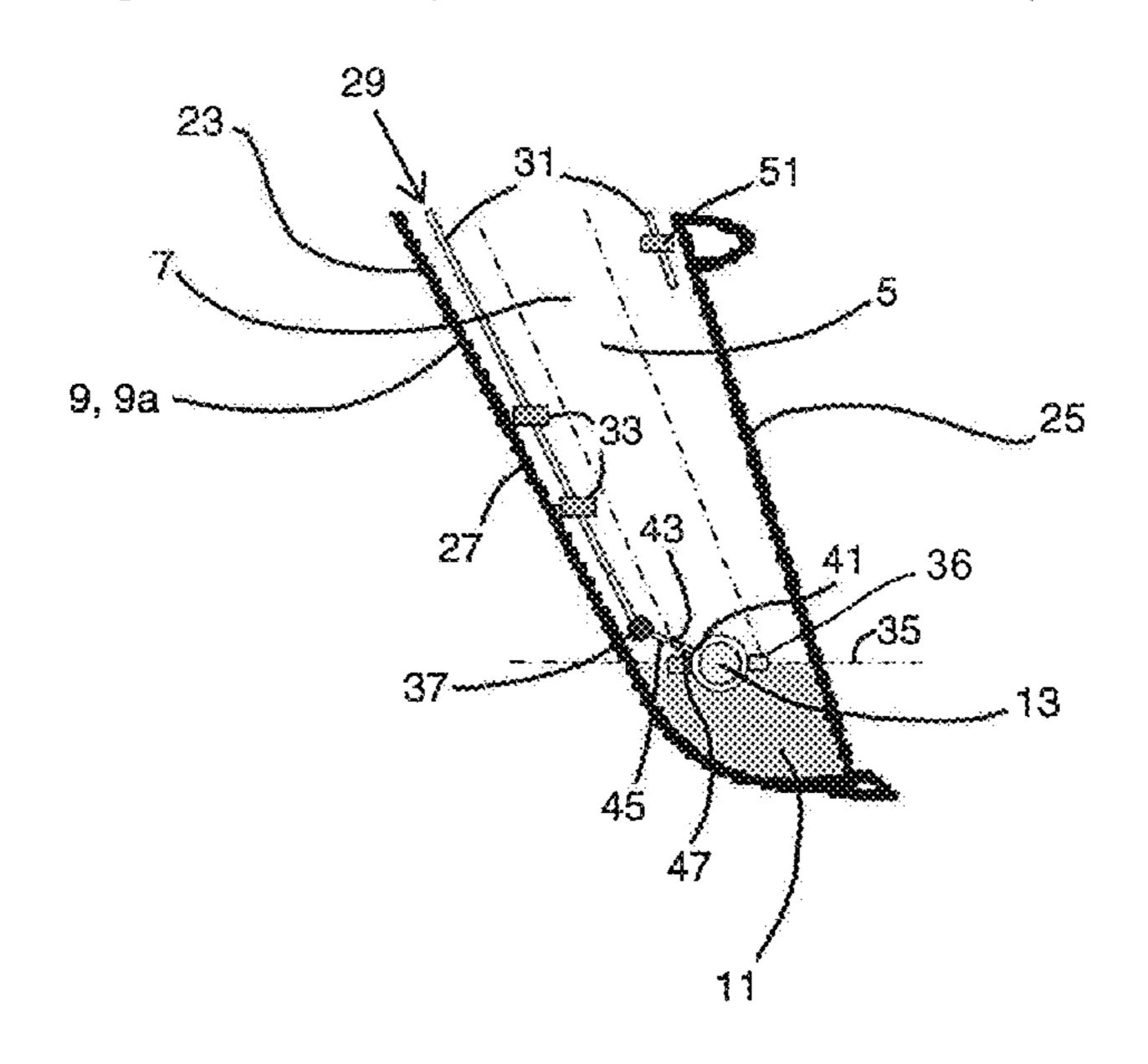
cost-efficient and light-weight wing, is achieved in that the high lift actuation system (29) is drivingly coupled to the tip actuation unit (13) to provide power to the tip actuation unit (13)
