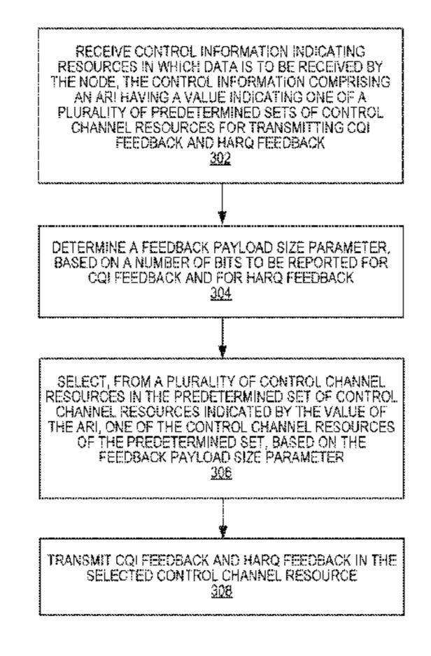
the feedback payload size parameter. The node transmits CQI feedback and HARQ feedback in the selected control channel resource.
