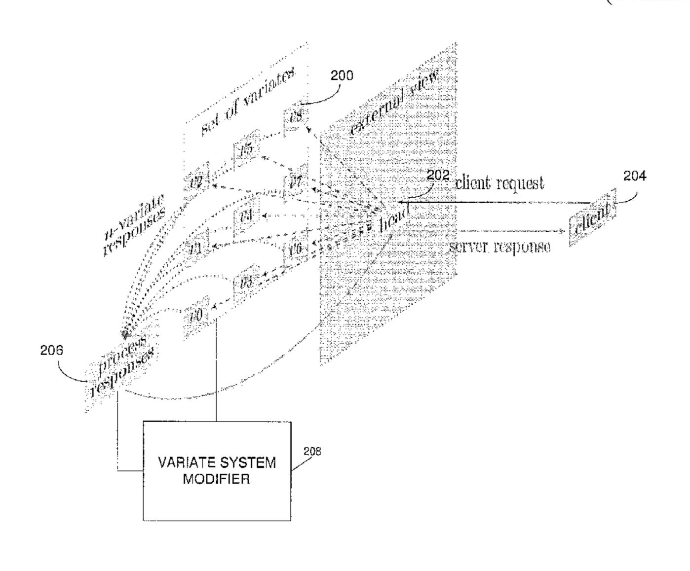
generate a response to the request. At least some of the variates are different in configuration from the other. The response processing server receives the responses from the variates, selects one of the responses, and delivers the response to the client via the head device. Configuration or systems diversity and adaptation to threats and failures over time may be achieved using adaptive algorithms.
