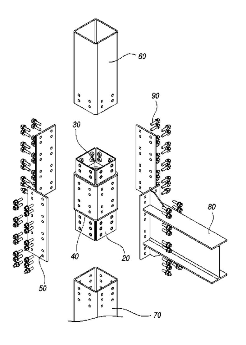
as compared with the related art, when a closed-section column and a beam are connected. Further, a closed-section column and a beam can be connected without welding, so the process can be shortened, connecting become easy, and quality is also uniform.
