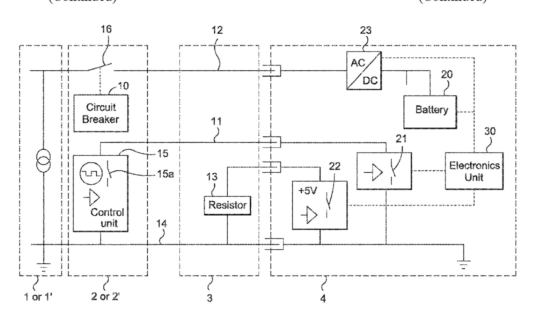
electronics unit detects physical parameters of the pilot signal via the pilot line, physical parameters of the power supply network at the power withdrawal point via the charging current lines, and physical parameters of the station charging device or of the cable charging device via the pilot line, respectively, during a charging process so as to produce a parameter data set characterizing the power withdrawal point.
