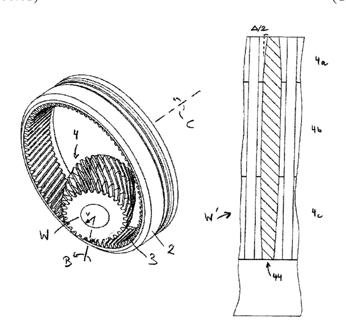
the machined toothed gearing with a tooth flank region (4a) of the machine tool gearing with tooth thickness increasing in the tooth trace direction from the end face (5) facing the machined toothed gearing.
