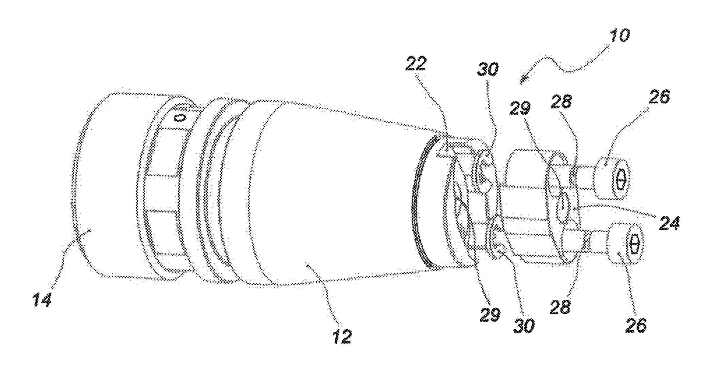
diameter rear part, into a complementary housing made in the rotating shaft of a motorised module. On the smaller diameter rear face of the tool holder shank a milling cut is made configured to accommodate at least one removable insert which protrudes partly frontally in the direction of a recess made on the back wall of the tapered seat of the rotating shaft of the motorized module.
