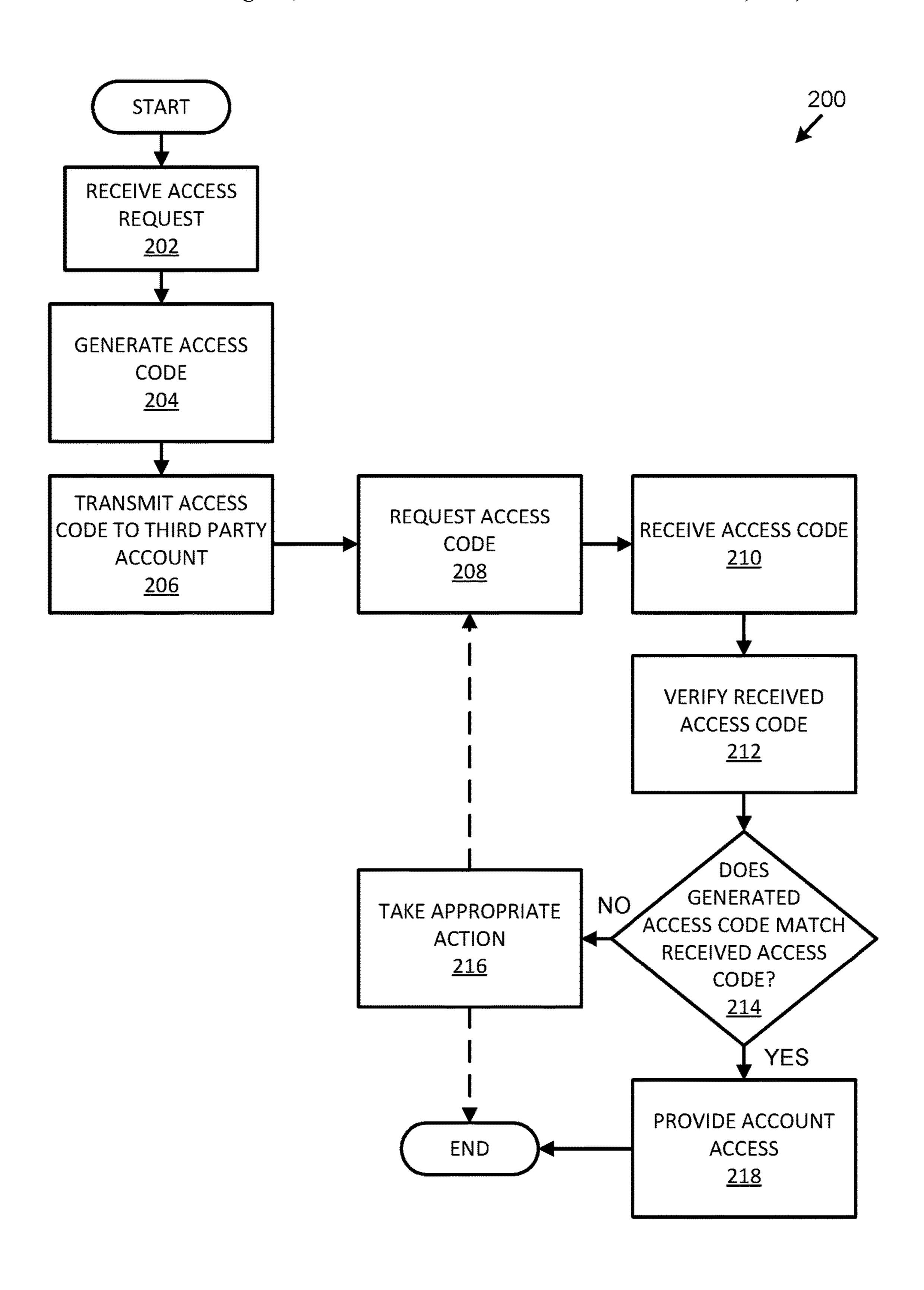
FIG 2: EXEMPLARY ACCOUNT ACCESS PROCESS – ACCOUNT SYSTEM PERSPECTIVE
