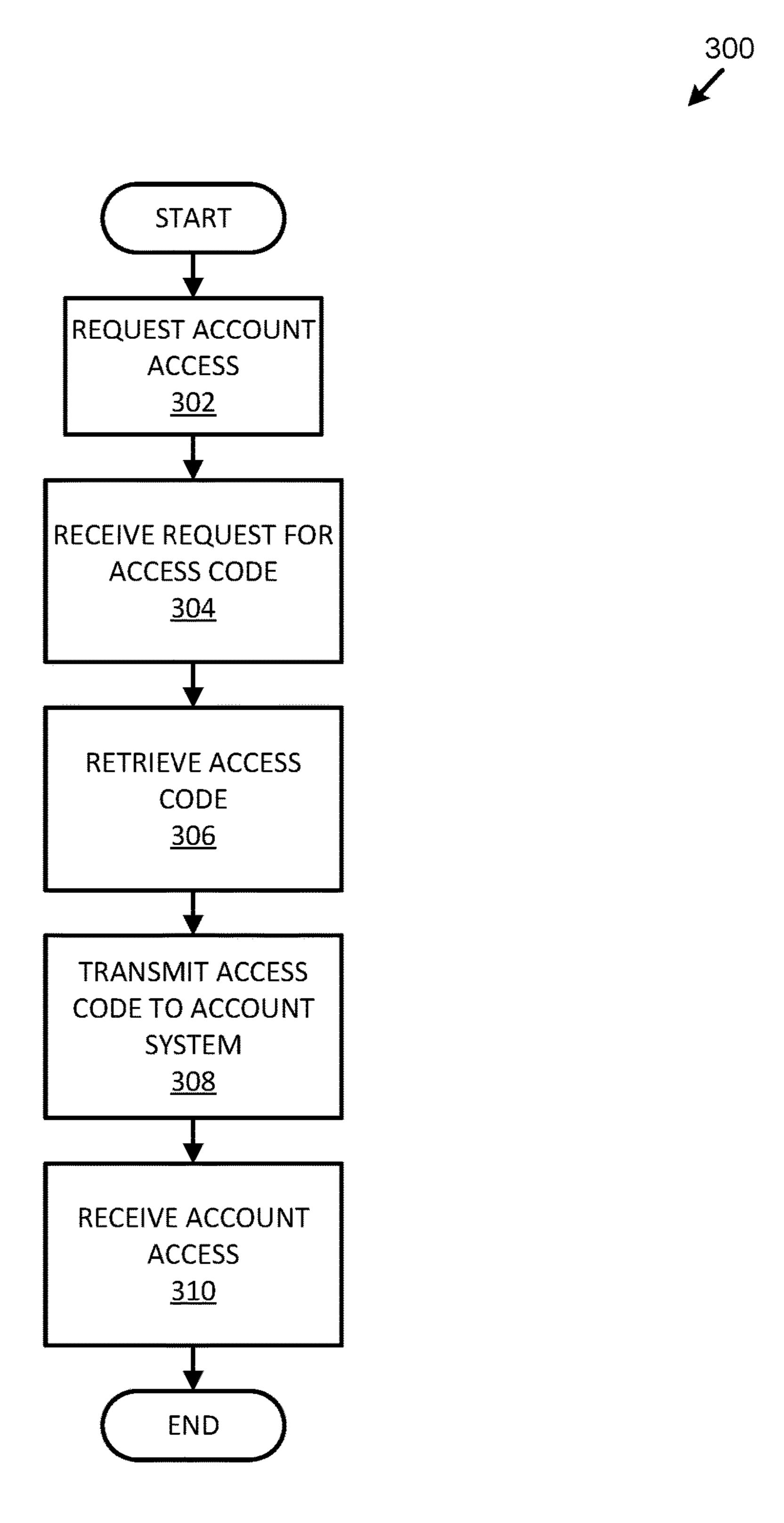
FIG 3: EXEMPLARY ACCOUNT ACCESS PROCESS – DEVICE PERSPECTIVE
