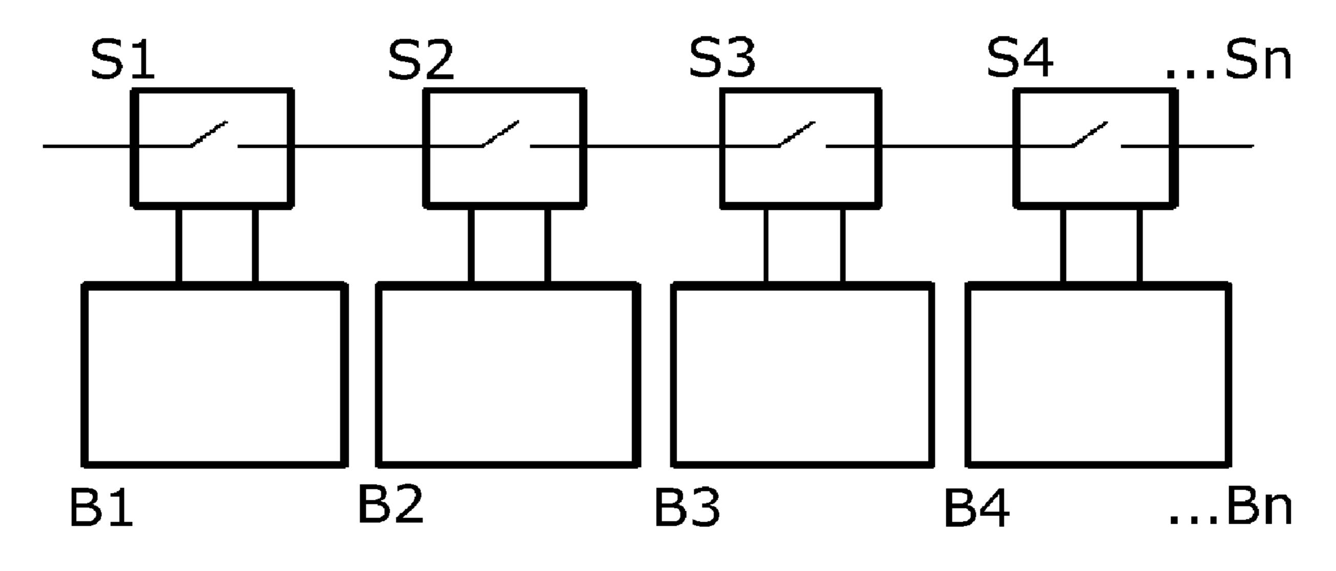
energy storage module. A total voltage is generated by at least two energy storage modules being activated with a time overlap but over activation periods of different length. One of the activation periods of different length is assigned to each of the at least two energy storage modules depending on the ascertained at least one power value.
