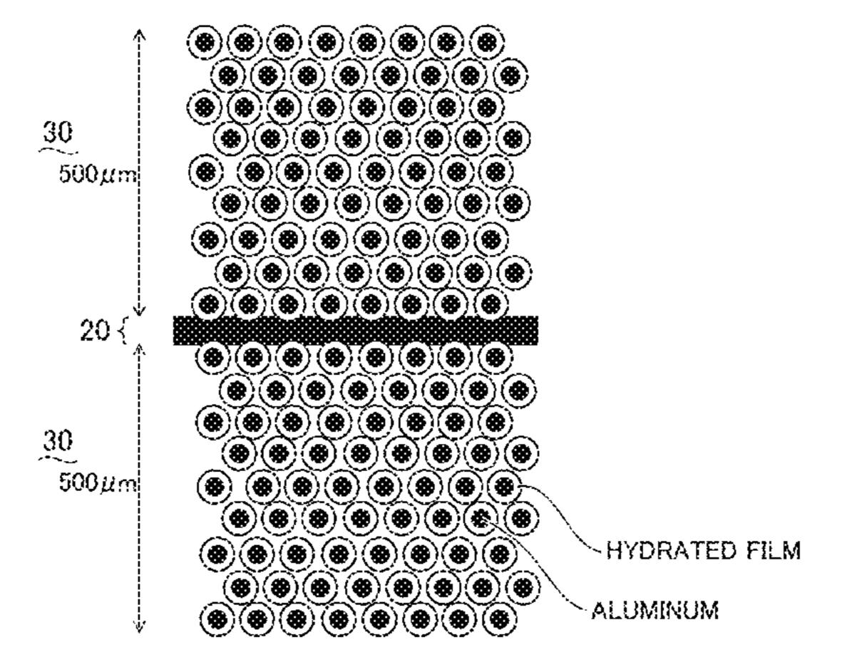
range of up to  $100~\mu m$  from the surface of the aluminum electrode, and t2 is the average thickness s of the hydrated film formed in a deep portion at least  $100~\mu m$  from the surface of the aluminum electrode.
