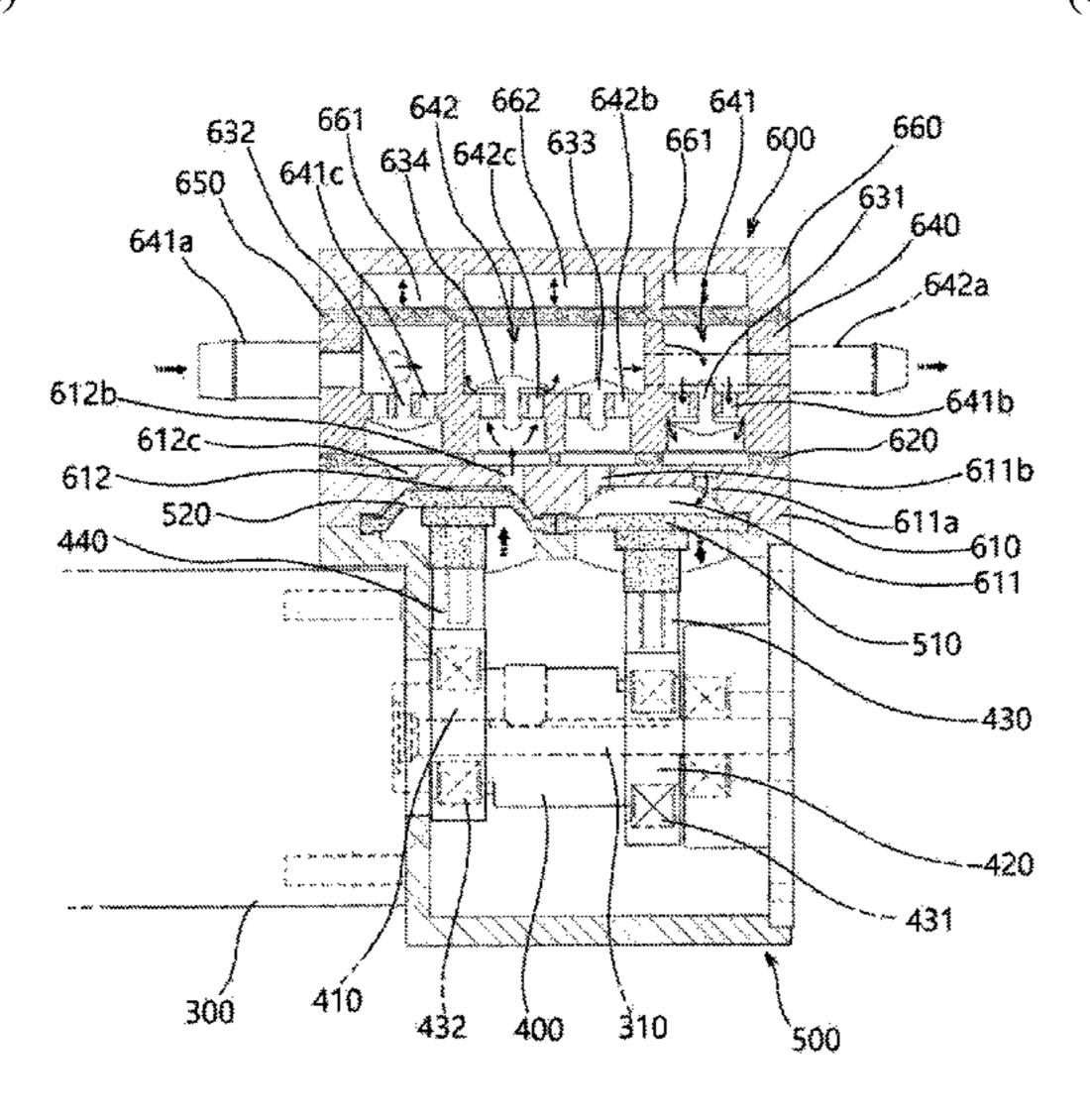
intake pressure and discharge pressure of fluid causes pressure balancing to occur.
