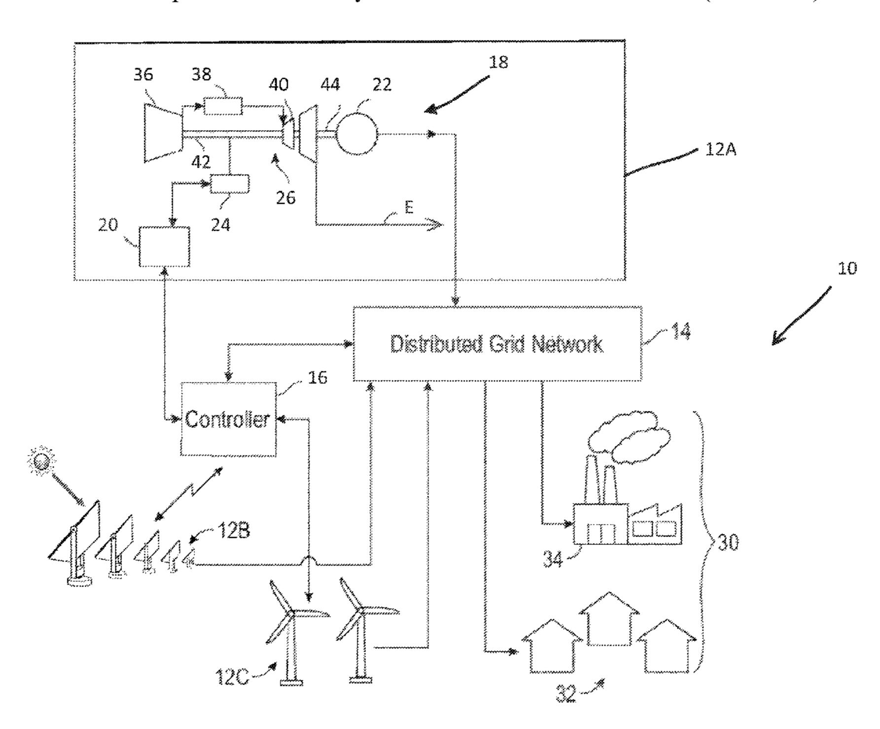
ate the generator as a starter-motor with power from: the first static frequency converter to turn the gas turbine engine at a first rate sufficient to start the gas turbine engine within a first time period or the first static frequency converter and the second static frequency converter in synchronization to turn the gas turbine engine at a second rate greater than the first rate.
