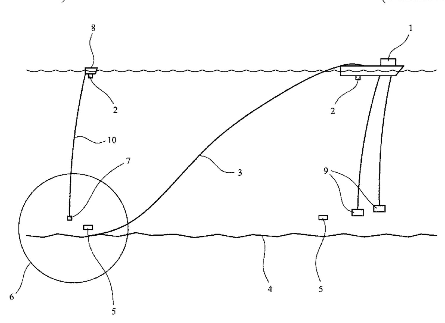
the unmanned underwater vehicle. The three communication arrangements are arranged in series such that, in use, the operator or observer may communication with the unmanned/autonomous underwater vehicle via the unmanned surface vessel, the wired connection between the unmanned surface vessel and the communication unit, and the wireless connection between the communication unit and the unmanned underwater vehicle.
