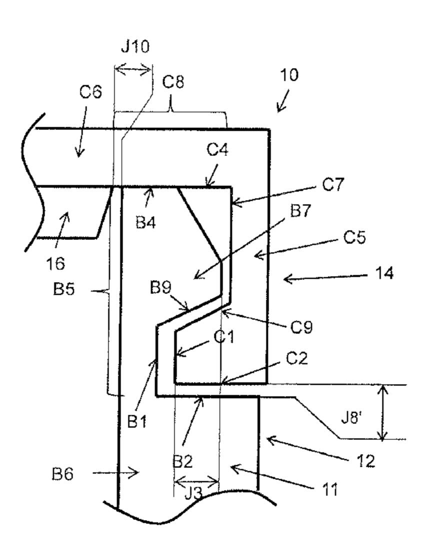
extension of the first portion of the peripheral body wall to form a gap between the step and the peripheral skirt.
