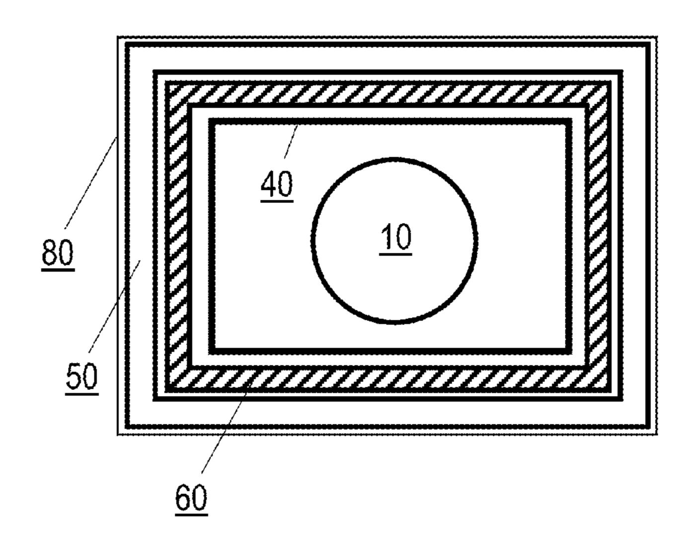
conversion by means of fission, fusion or aneutronic nuclear reactions and for generating electric energy, wherein the reactor contains a neutron elimination device (50) which contains tin and is arranged such that at least some moderated neutrons are made to undergo a nuclear reaction with the tin.
