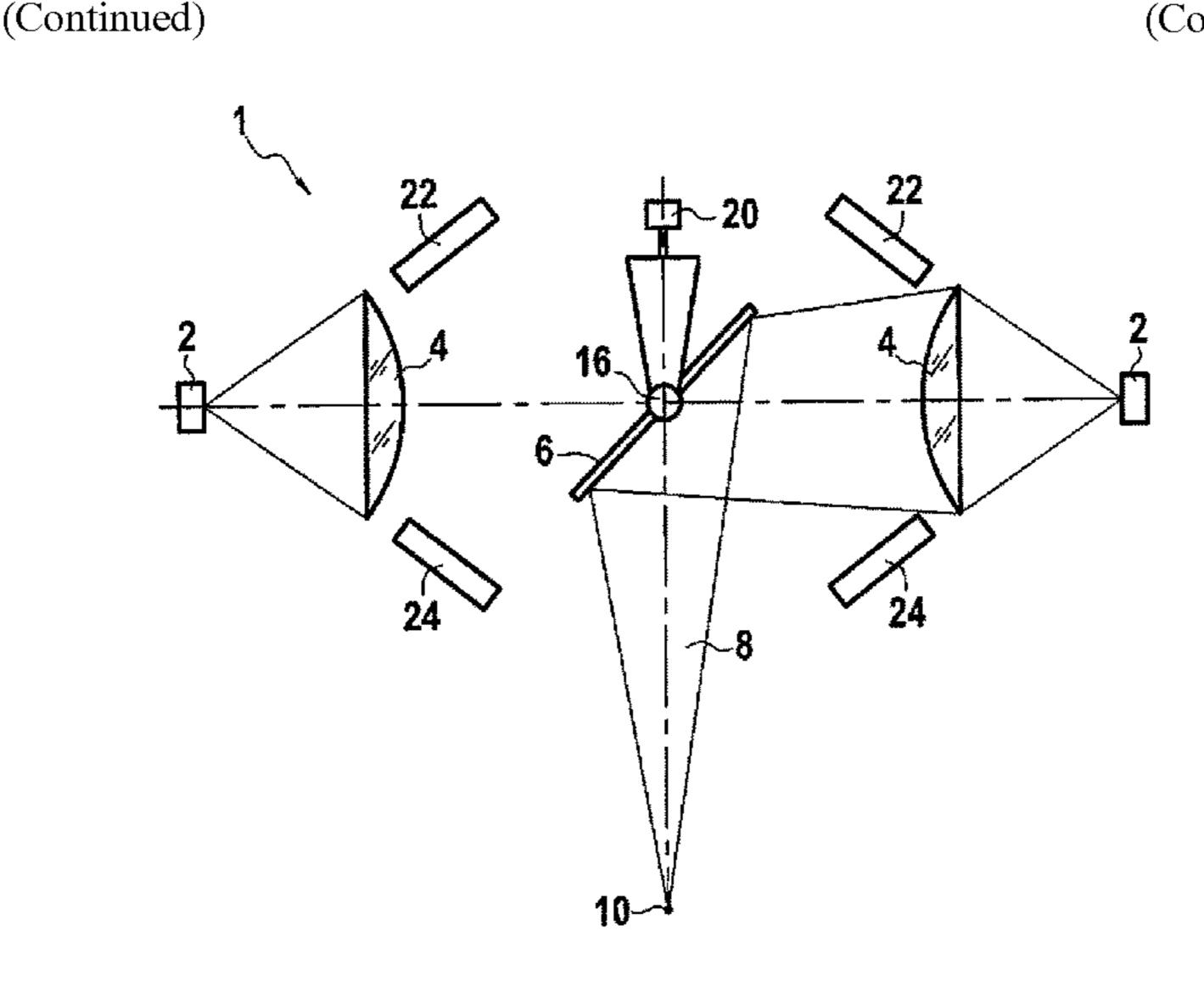
In particular, the reflector means (6) are mounted to move in the detection zone of each microwave sensor (2) in such a manner as to move said detection zone by moving the reflector means (6). The invention also provides a corresponding microwave imaging method.
