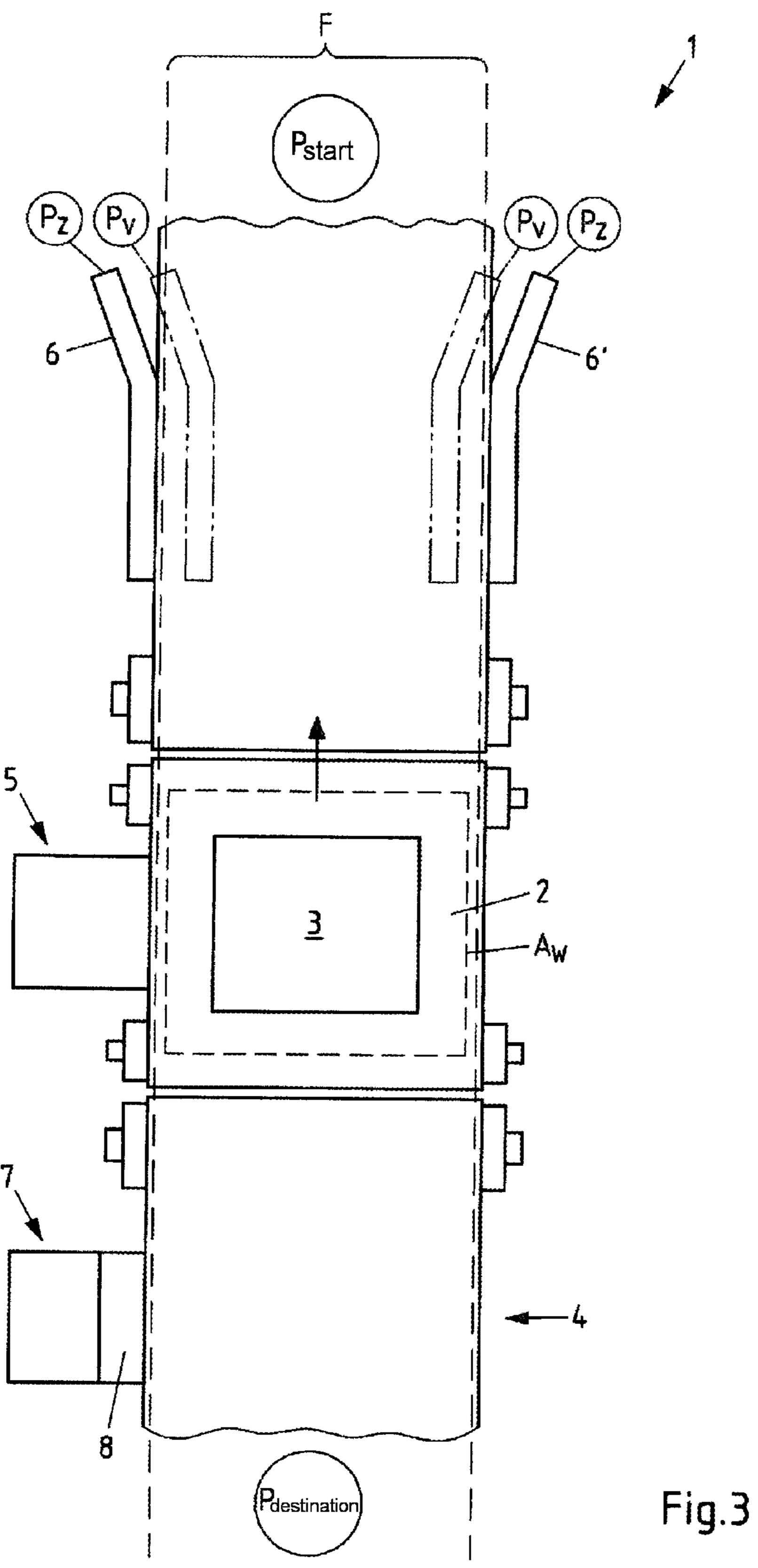
DEVICE AND METHOD FOR WEIGHING A PRODUCT IN A WEIGHING SECTION THAT INCLUDES A CONVEYING DEVICE FOR TRANSPORTING THE PRODUCT IN A DIRECTION FROM A START POSITION OVER THE WEIGHING SECTION TO A DESTINATION POSITION AND A CONTROL **DEVICE CONFIGURED TO** AUTOMATICALLY STOP THE CONVEYING DEVICE DURING ITS OPERATION TO ACHIEVE A STOPPED STATE AND THEN TO AUTOMATICALLY OPERATE THE CONVEYING DEVICE IN A REVERSE MOVEMENT DIRECTION UNTIL THE PRODUCT IS NO LONGER LOCATED IN THE WEIGHING SECTION
