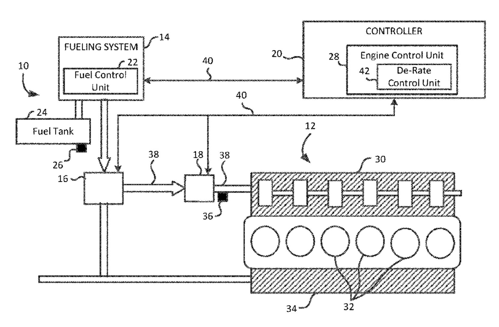
de-rate operation on the engine (12) by adjusting one or more operational parameters related to an engine (12) load based on the detected low fuel condition. De-rate condition monitoring unit (208) monitors the detected low fuel condition for a predetermined time period in response to the operational parameter adjustment performed by operational parameter adjustment unit (206).
