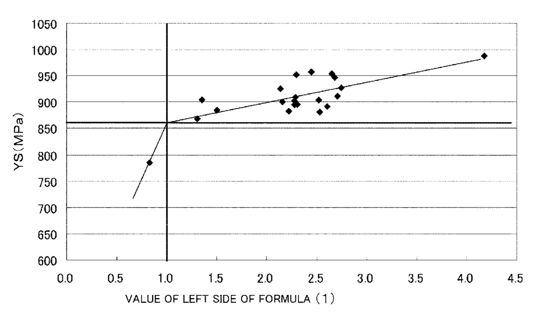
3.0% or more and less than 5.0%, W: 0.1 to 3.0%, Nb: 0.07 to 0.5%, V: 0.01 to 0.5%, Al: 0.001 to 0.1%, N: 0.010 to 0.100%, O: 0.01% or less, and Fe and unavoidable impurities as a balance. Nb, Ta, C, N and Cu satisfy a specified formula. The steel pipe has a microstructure which is formed of 45% or more of a tempered martensite phase, 20 to 40% of a ferrite phase, and more than 10% and 25% or less of a residual austenite phase in terms of volume ratio.
