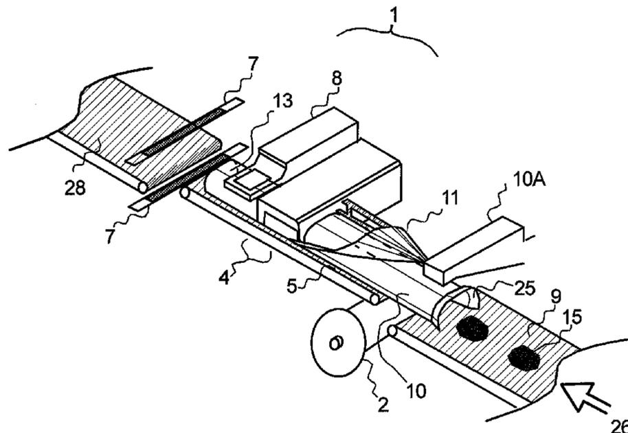
forming tube. Data may be printed on an upper film surface over a platen including an upper part of the forming tube. An outfeed conveyor carries transversely sealed wrapped items on to a vacuum sealer.
