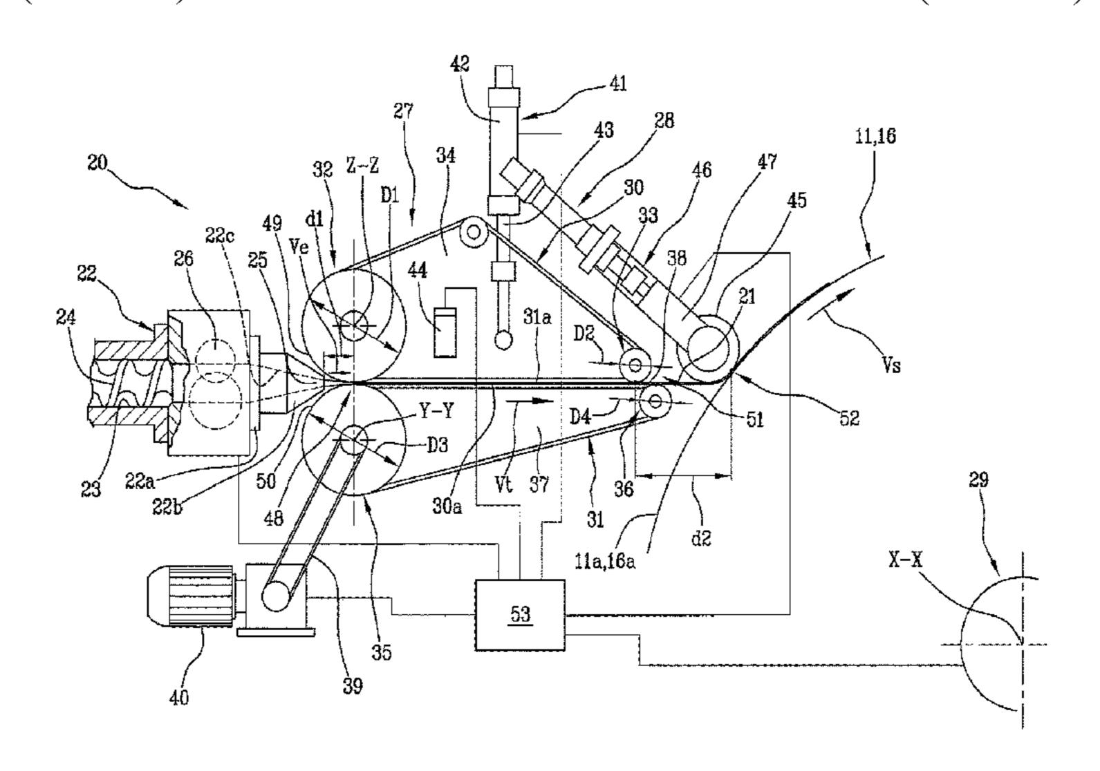
stretched with a supplementary stretch coefficient greater than the first stretch coefficient, in a manner so as to confer, also to the span adjacent to the head end, a stretch and a section similar or substantially equivalent to those of the rest of the continuous elongated element.
