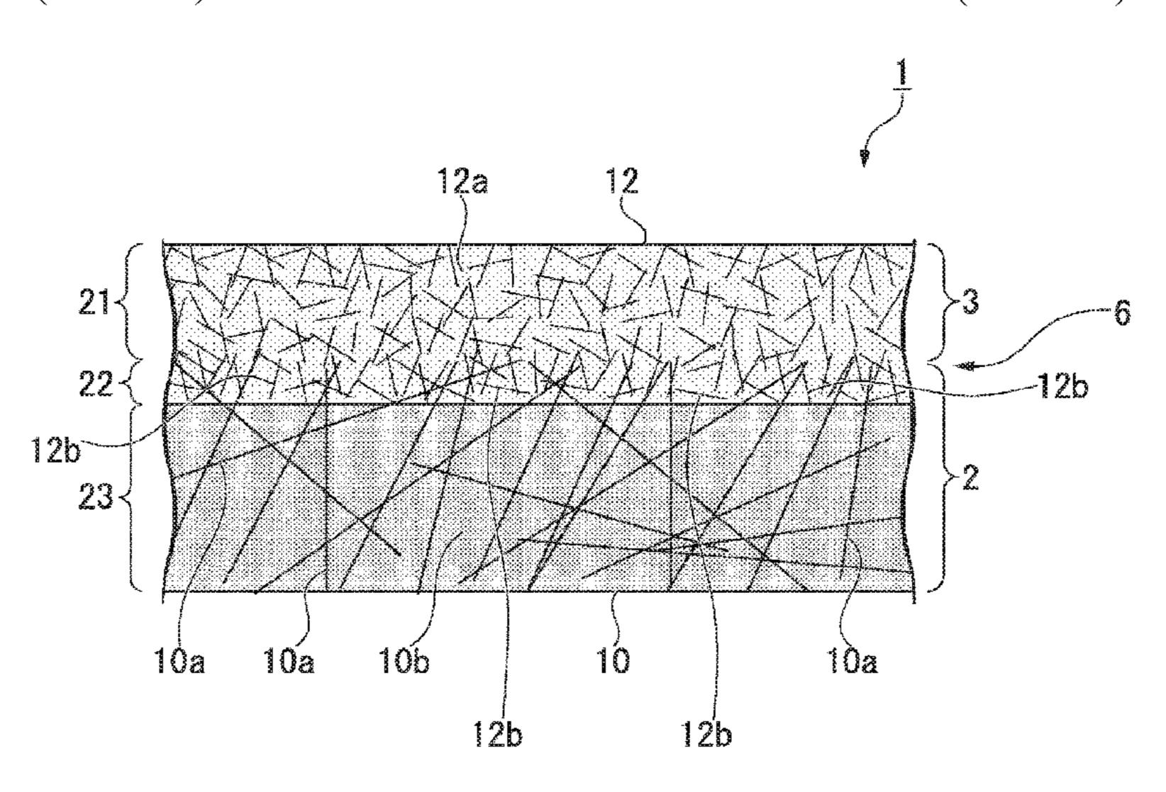
(y2) having a fiber length of 0.02 mm to less than 3 mm with respect to the total volume of reinforcing fibers present in the layer, and the volume content of fibers in each layer being controlled so as to be in specific ranges.
