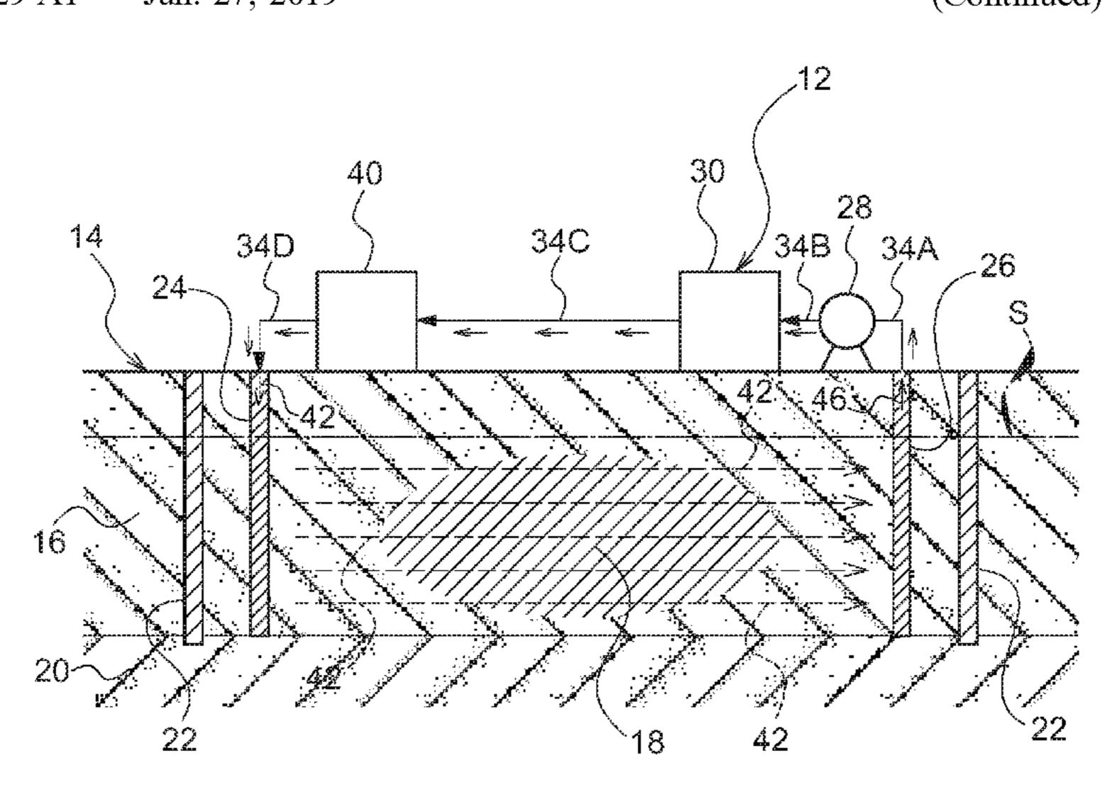
perature, into an injection well provided in the ground, and a second process of pumping up groundwater containing the cleaning liquid, in which the contaminant separated from the subsurface soil has been dissolved, from a pumping well that is provided in the ground so as to be spaced apart from the injection well.
