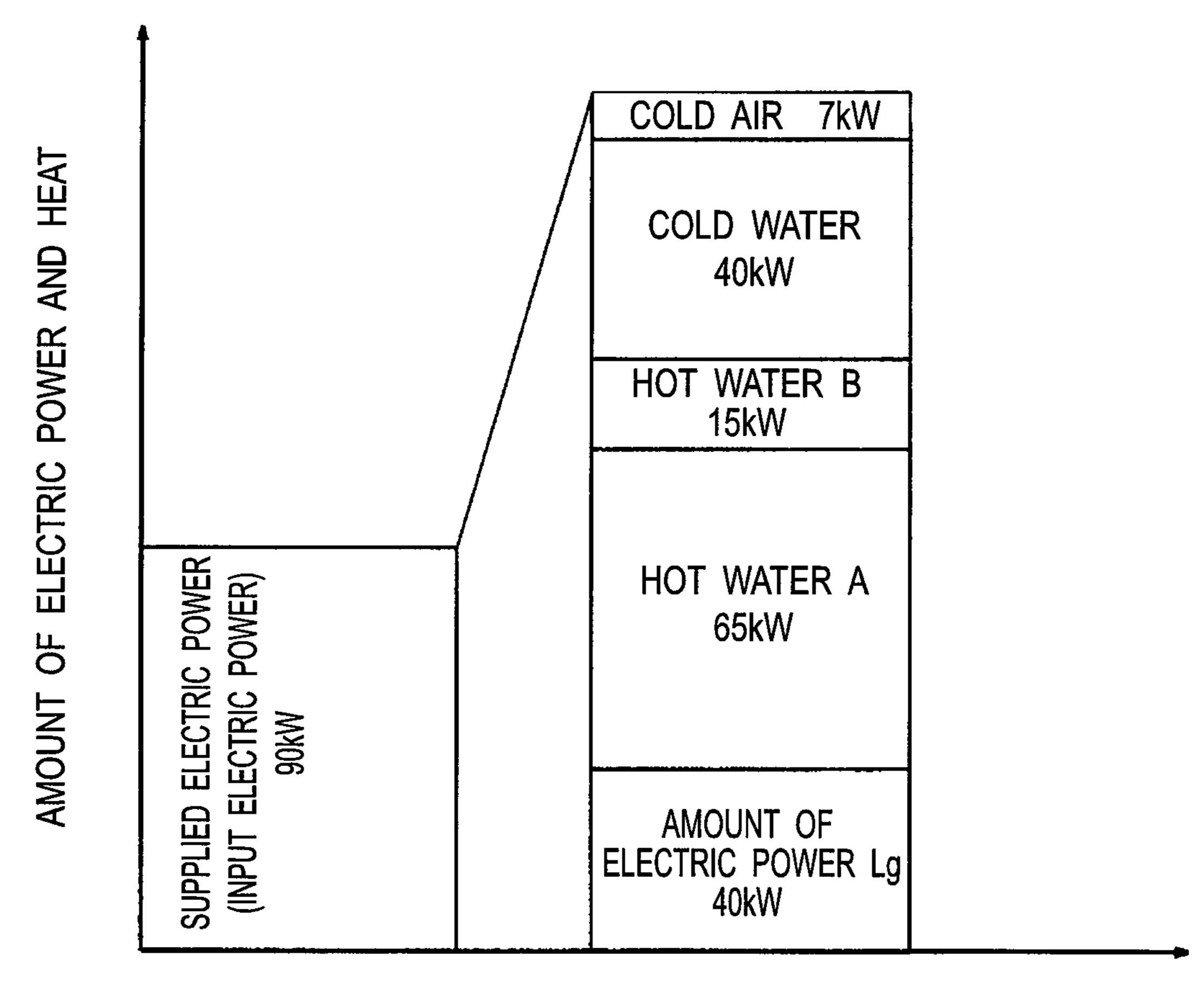
OPERATION MODE IN WHICH HEATING AND COOLING AND POWER GENERATION ARE BOTH PERFORMED
