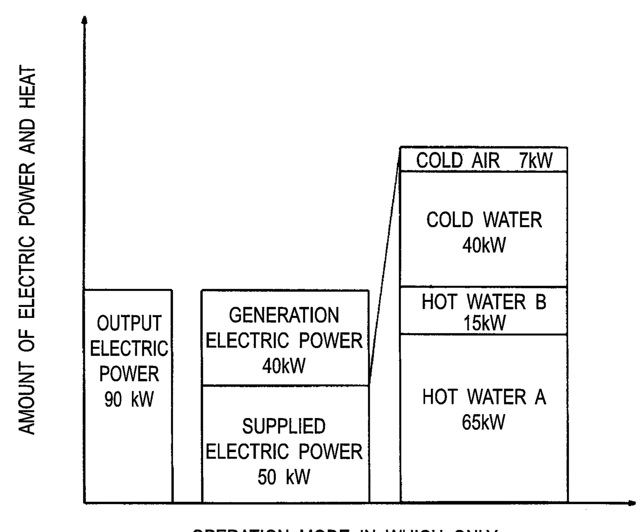
OPERATION MODE IN WHICH ONLY HEATING AND COOLING IS PERFORMED
