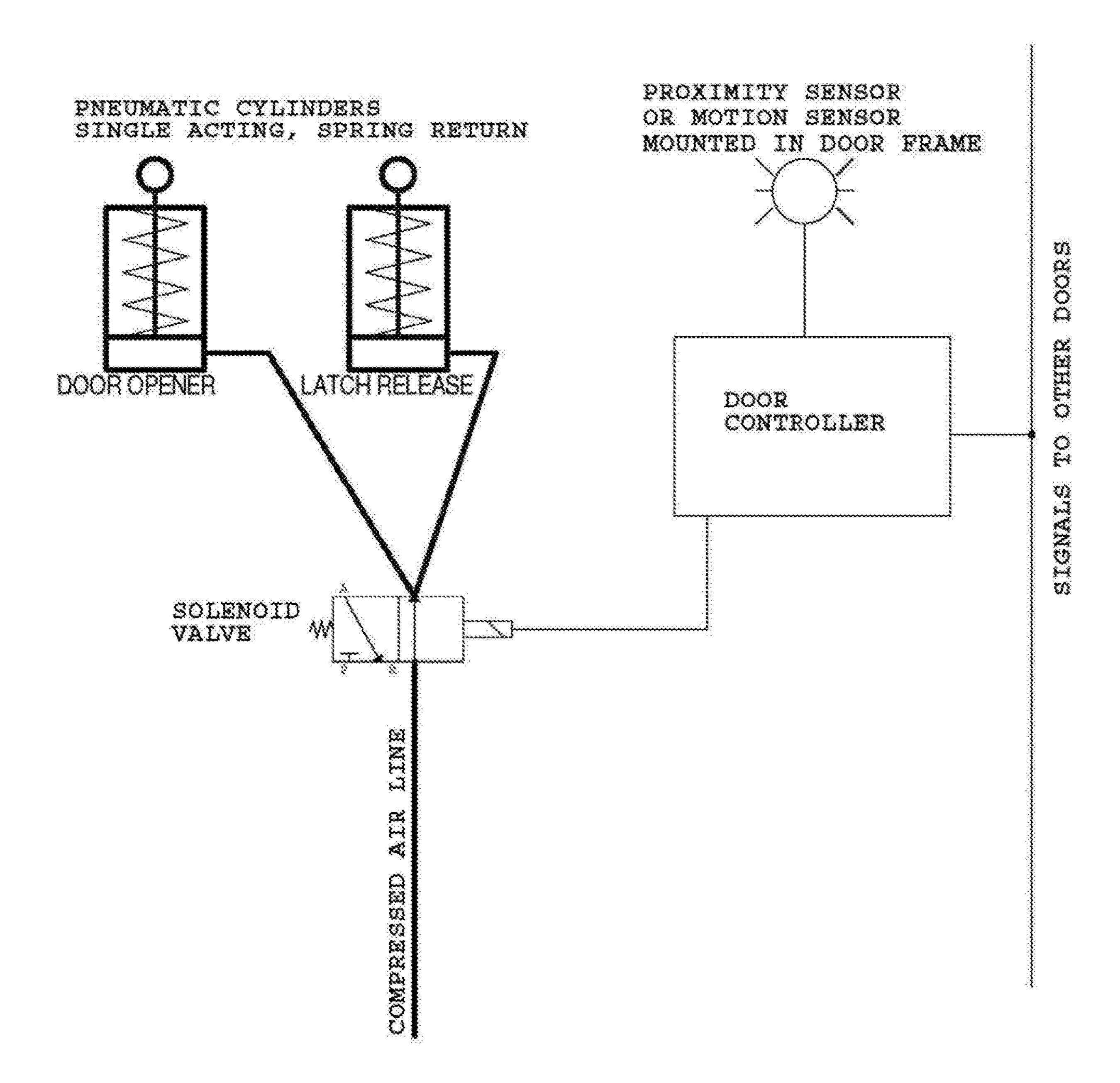
DOOR CONTROLLER DETECTS PERSON VIA SENSOR AND THEN INITIATES DOOR OPEN CYCLE
