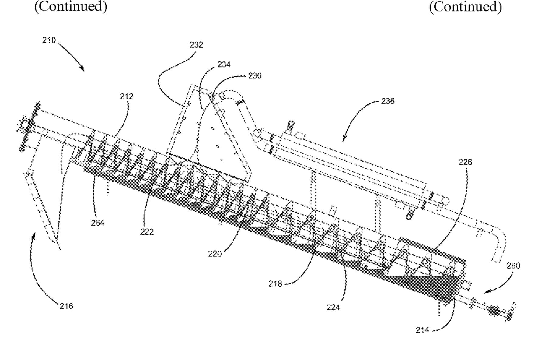
and discharging from the housing, separately to the extracting of the airflow from the housing, the sludge from which the moisture has been removed.
