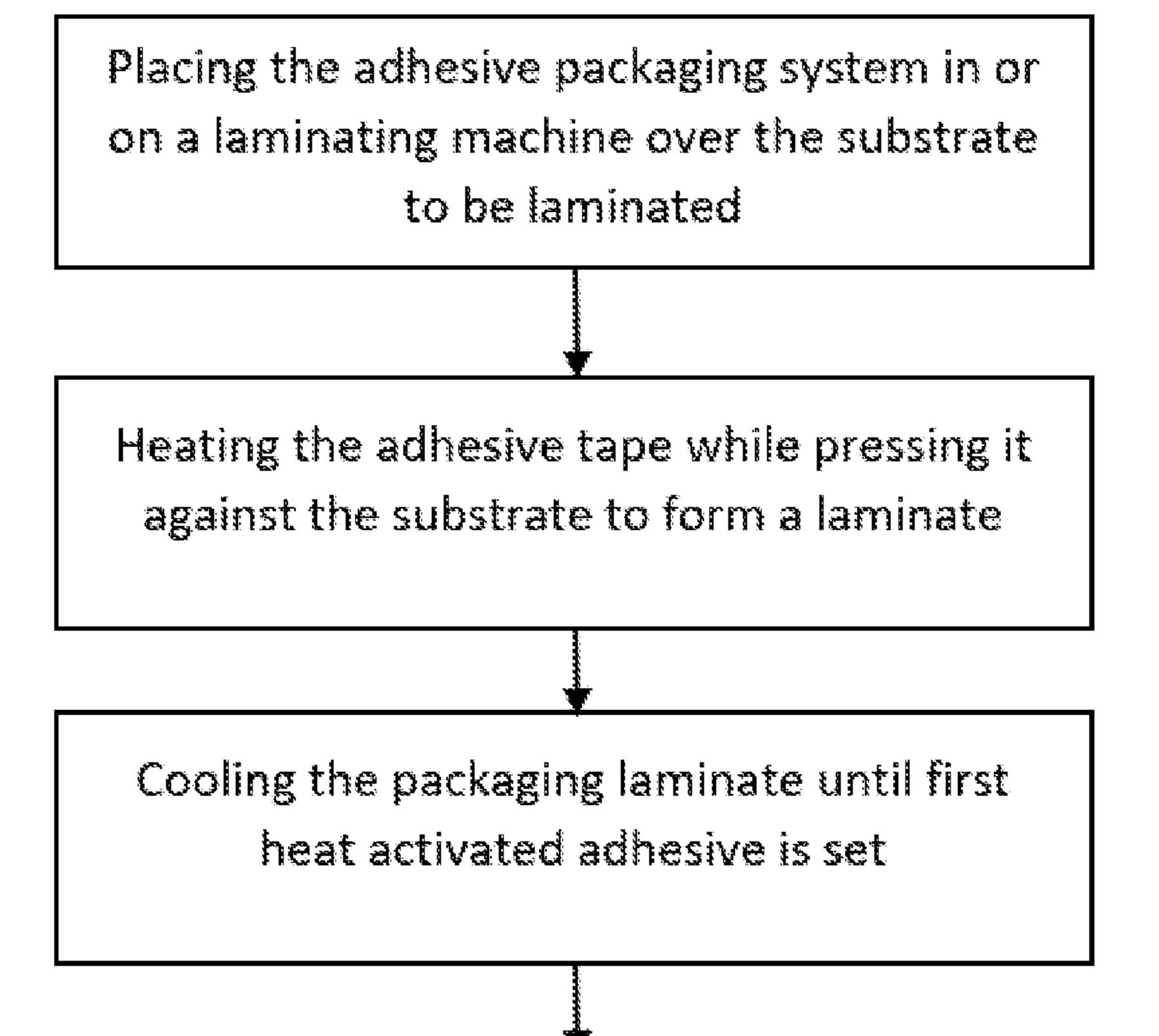
Cutting a predetermined portion of the packaging laminate before a second adhesion occurs between the tape and the packaging laminate when the second heat activated adhesive is set
