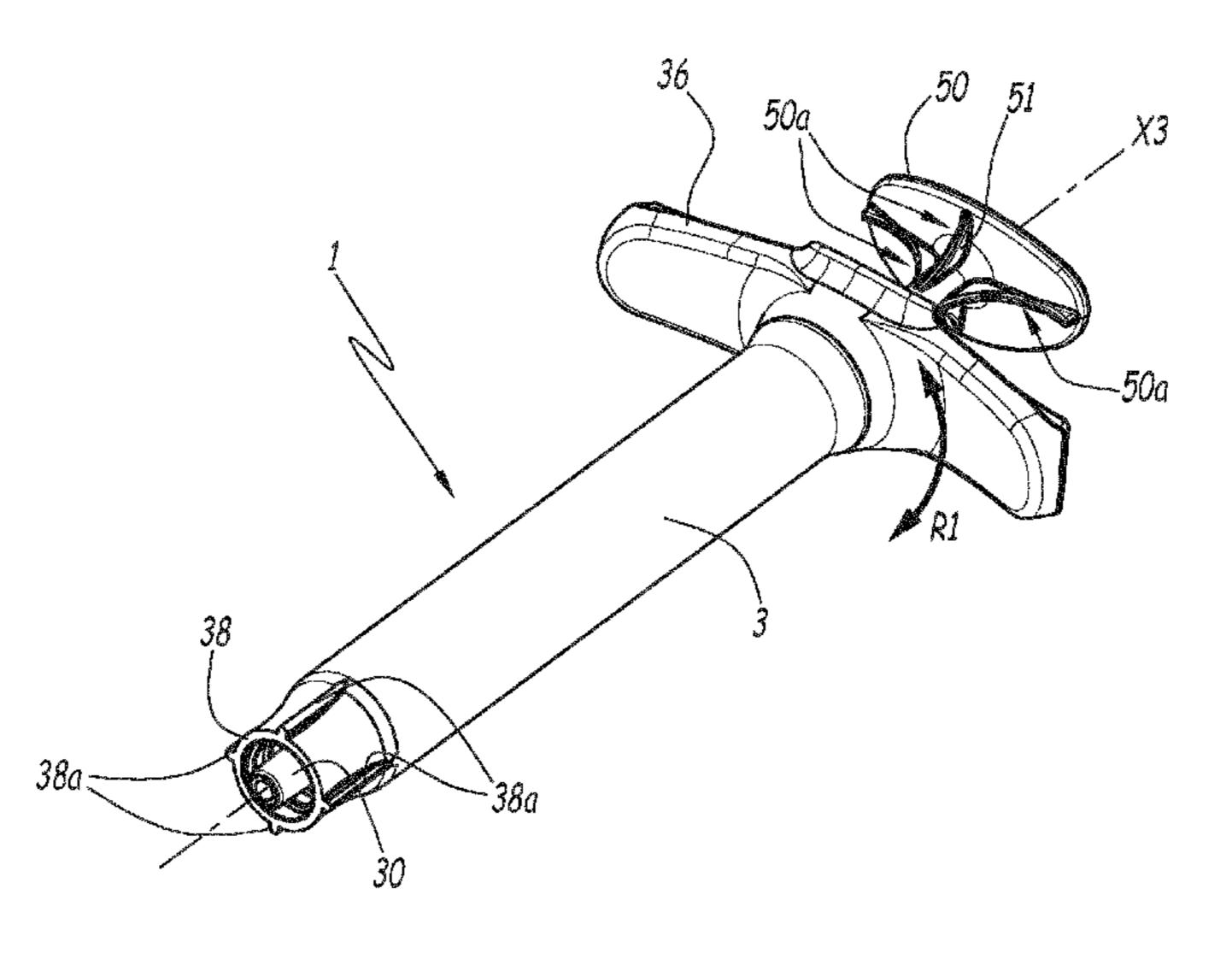
gripping members (34, 36) provided on the body (3). The piston (5) is formed from a single piece made from a material having a Young's modulus greater than 3000 MPa and the piston (5) has no elastic area between the gripping member (50) of same and the substance to be injected.
