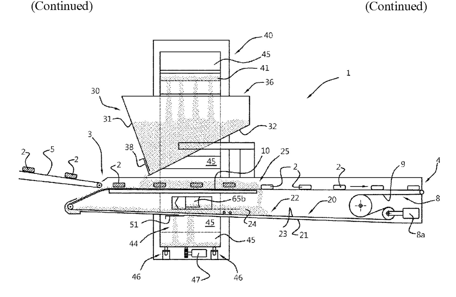
controls a discharge opening in the recovered excess coating material bed support. An adjustable upper layer diverter device engages an upper layer of the recovered excess coating material bed passing over the recovered excess coating material bed support and diverts at least a portion of the upper layer at an adjustable rate into the particulate coating material elevator device.
